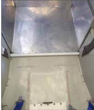
Location for the auxiliary tank platform in the RV-8 passenger area.
