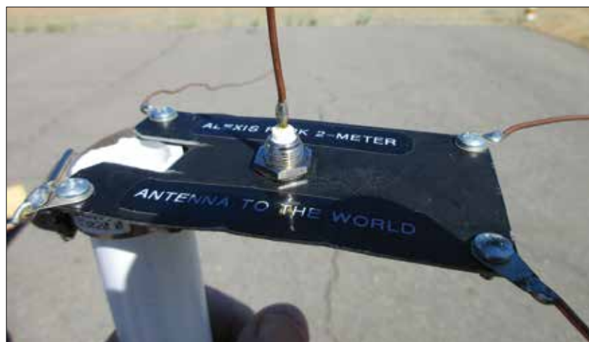
Close-up of the construction detail of the vertical radiating element, the four horizontal ground plane elements, and the black aluminum mounting base.
