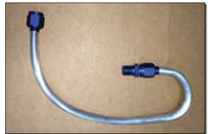
Fabricated fuel line between the fuel selector and the quick-disconnect.
