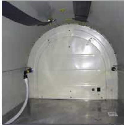
Vent hose connection in aft baggage compartment.
