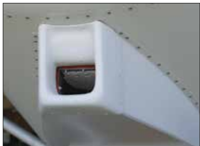
Collin made this custom lower cowl fairing to feed the Van's filtered air box.
