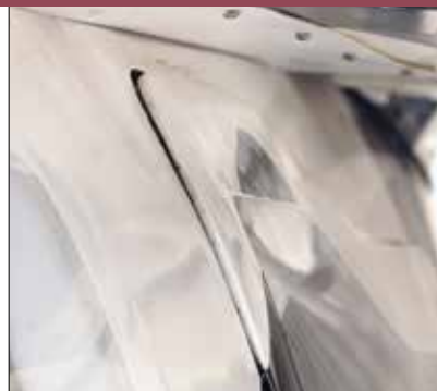
(Left) The cargo door without the doorjamb doodad. (Right) The doodad draws the door flush. I'm told that subsequent to my kit, Jabiru changed the hinge design to resolve this issue.
