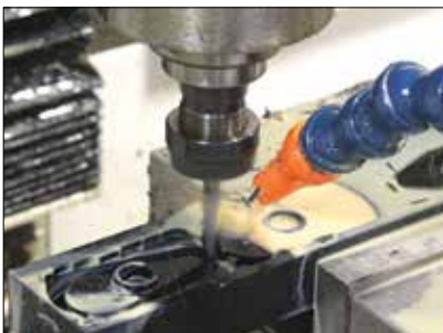
(Left) Profiling the backside lip of the doodad and milling the outside profile. Delrin machines beautifully, but is sensitive to spindle speeds and feed rates. Too much of one and too little of the other can easily melt the material. Flood coolant on the CNC machine allows for more aggressive speeds and feeds. (Center and Right) Using a band saw to cut the first operation from the 2-inch x 1-inch rectangle bar milling stock.
