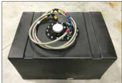
Auxiliary tank with attached fuel and vent hoses.
