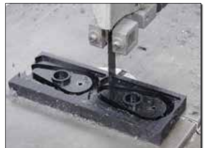
(Left) Profiling the backside lip of the doodad and milling the outside profile. Delrin machines beautifully, but is sensitive to spindle speeds and feed rates. Too much of one and too little of the other can easily melt the material. Flood coolant on the CNC machine allows for more aggressive speeds and feeds. (Center and Right) Using a band saw to cut the first operation from the 2-inch x 1-inch rectangle bar milling stock.
