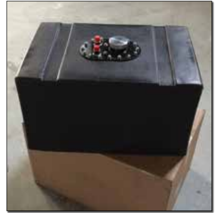
Twenty-two gallon circle track fuel cell.
