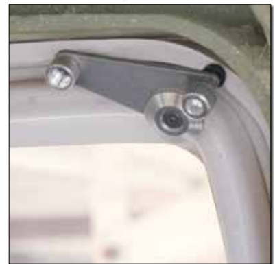
Inside cabin view of the doorjamb doodad with the lever open (left) and engaged for flight (right). The tensioning screw adjusts the door in or out as needed, to bring it flush with the fuselage.
