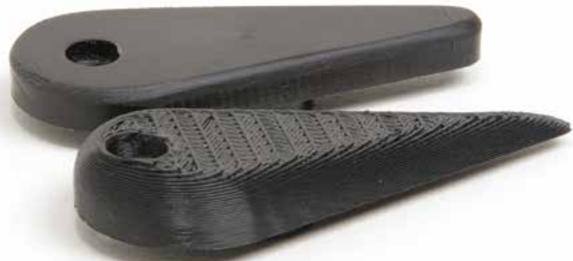
This close-up shows the difference in shape and surface finish between the machined part (top) and the 3D printed part. Note the 3D printed doodad is tapered front to back.
