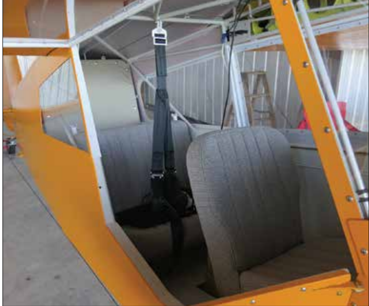
(Left) Oil temperatures were high before Collin added this filter and cooler adapter from Steve's Aircraft. (Right) The Bearhawk LSA interior looks a lot like the Bearhawk Patrol in dimensions. Collin left the interior unfinished to save weight in the LSA.
