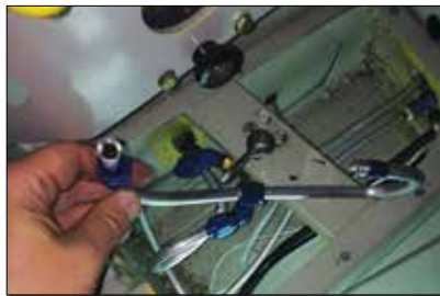
Fabricated fuel line oriented for installation.
