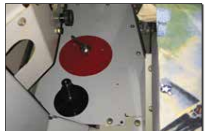
Completed quick-disconnect is located near the fuel selector.
