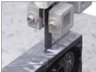
(Left) Profiling the backside lip of the doodad and milling the outside profile. Delrin machines beautifully, but is sensitive to spindle speeds and feed rates. Too much of one and too little of the other can easily melt the material. Flood coolant on the CNC machine allows for more aggressive speeds and feeds. (Center and Right) Using a band saw to cut the first operation from the 2-inch x 1-inch rectangle bar milling stock.
