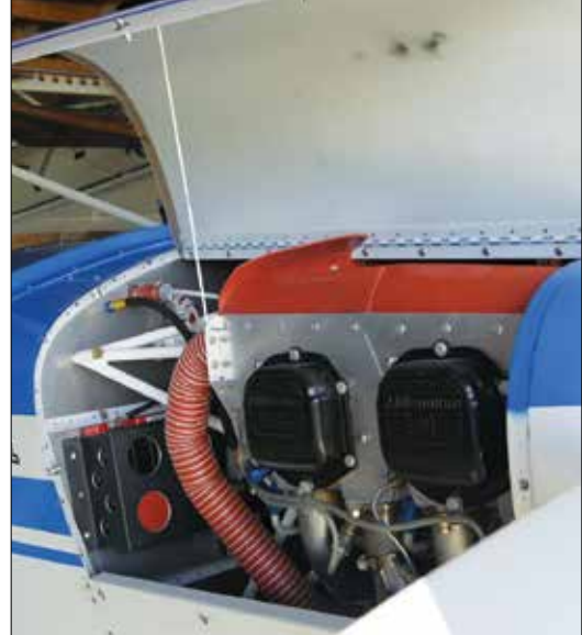
(Left) The Bearhawk Patrol is shaped like several other airplanes in its class, but it is one of the fastest among them. (Right) With a cowl that opens this far, preflight inspections can be much more complete, and minor maintenance is faster. Swapping out a fouled plug takes minutes.
