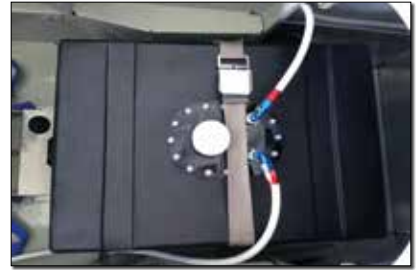
Auxiliary tank installed in the RV-8 passenger area.
