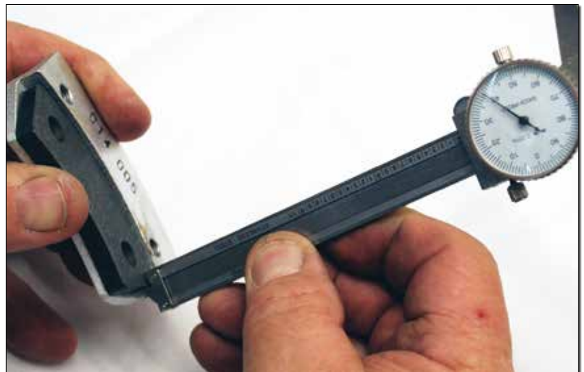
The depth rod of a dial caliper is used to check the thickness of a brake pad. This new pad measures .240 inches thick. When it gets down to .125 inch it will need to be replaced.
