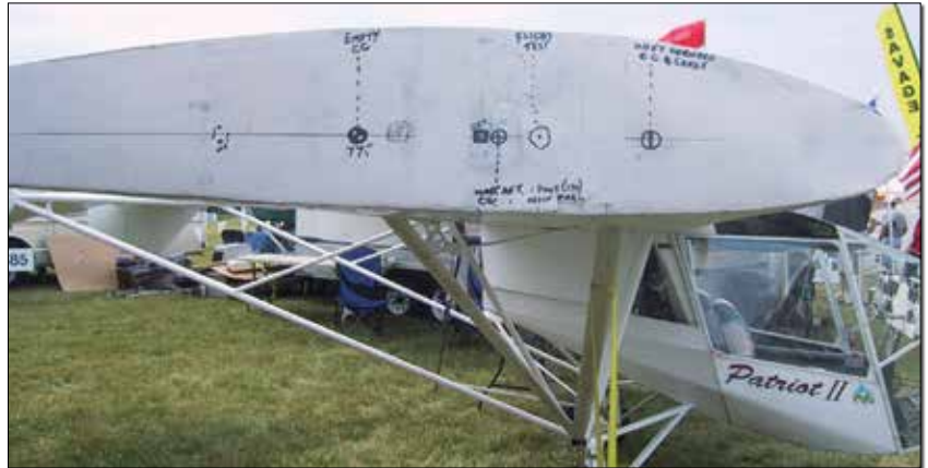
During flight testing of this prototype LSA, they actually marked the CG positions on the outboard wing tip rib.
