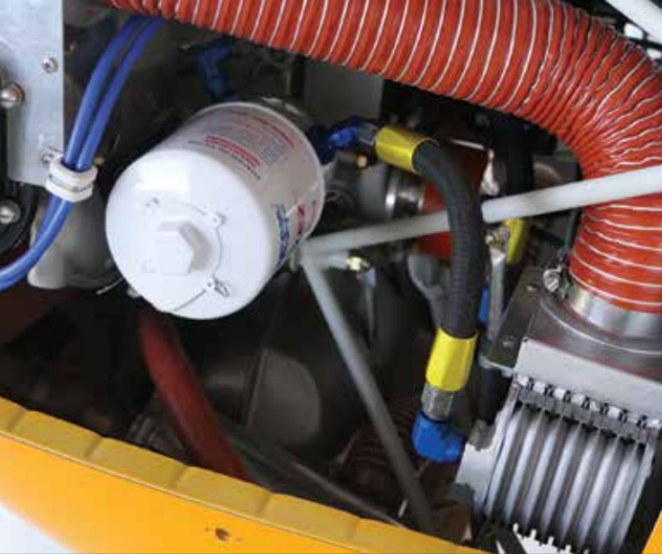
(Left) Oil temperatures were high before Collin added this filter and cooler adapter from Steve's Aircraft. (Right) The Bearhawk LSA interior looks a lot like the Bearhawk Patrol in dimensions. Collin left the interior unfinished to save weight in the LSA.
