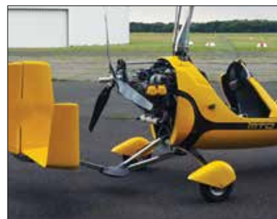
Ivoprop ground-adjustable prop.
