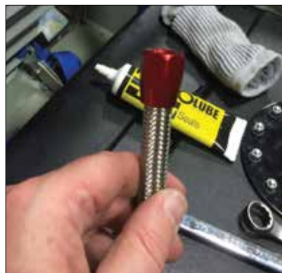
Half of the hose end fitting attached to braided fuel hose.
