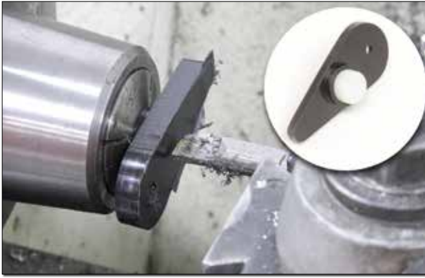
(Left) A plastic rod pressed into the counterbore (inset) provides a hold for the collet in order to face turn the doodad to the desired thickness. (Right) The edges were rounded over with a file and then polished with fine-grit sandpaper.
