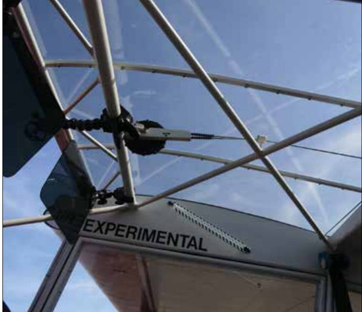
(Left) The panel is familiar and reliable, with a recently added Stratus ESG transponder for ADS-B Out. (Right) The sunshades are from RAM, the same folks that make mounts for electronic gadgets. The large skylight opens up the feeling of the cabin and makes the horizon visible in steep turns. Fuel sight gauges are simple and reliable. The elevator trim system is overhead.
