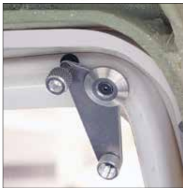
Inside cabin view of the doorjamb doodad with the lever open (left) and engaged for flight (right). The tensioning screw adjusts the door in or out as needed, to bring it flush with the fuselage.
