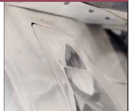
(Left) The cargo door without the doorjamb doodad. (Right) The doodad draws the door flush. I'm told that subsequent to my kit, Jabiru changed the hinge design to resolve this issue.
