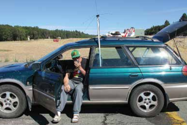
(Left) A typical airport setup for emergency communications at KGOO. The antenna is fastened to a PVC pipe and held in place by the left rear window. In the background you can see the S2 fire bomber aircraft. (Right) Close-up of the antenna. This one is around ten years old and about ready for a rebuild.
