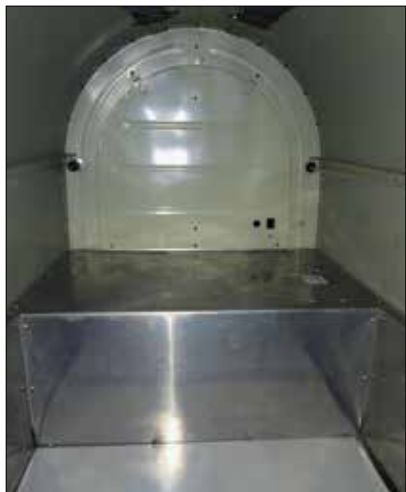
Auxiliary tank platform and vent hose quick-disconnect plug.
