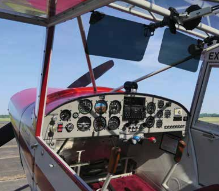
(Left) The panel is familiar and reliable, with a recently added Stratus ESG transponder for ADS-B Out. (Right) The sunshades are from RAM, the same folks that make mounts for electronic gadgets. The large skylight opens up the feeling of the cabin and makes the horizon visible in steep turns. Fuel sight gauges are simple and reliable. The elevator trim system is overhead.
