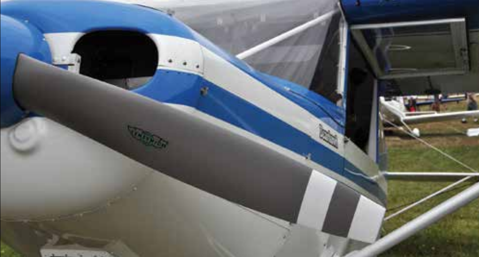
Sensenich fixed-pitch aluminum prop on a Bearhawk.
