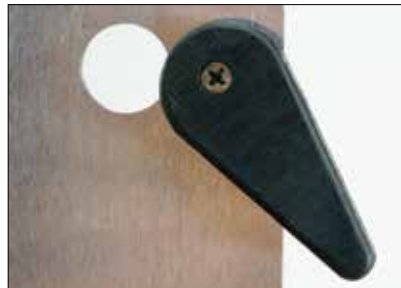
(Left and Center) Adjust the pivot screw so it's flush with the face of the doodad with the cover closed. If the screw is too tight or the counterbore too shallow, you won't be able to lift the cover and pivot it clear of the hole. (Right) A cross-section view of the test assembly with the doodad in the open position.
