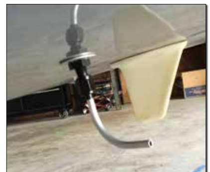
Finished vent line on the bottom of the fuselage.
