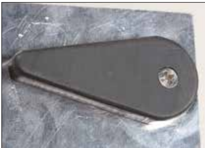
(Left and Center) Adjust the pivot screw so it's flush with the face of the doodad with the cover closed. If the screw is too tight or the counterbore too shallow, you won't be able to lift the cover and pivot it clear of the hole. (Right) A cross-section view of the test assembly with the doodad in the open position.
