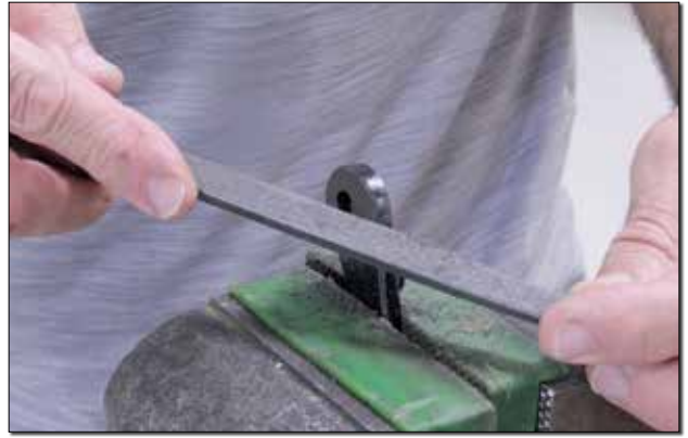
(Left) A plastic rod pressed into the counterbore (inset) provides a hold for the collet in order to face turn the doodad to the desired thickness. (Right) The edges were rounded over with a file and then polished with fine-grit sandpaper.
