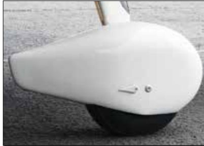
(Left) The teardrop protrusions on the sides of the wheel pants are spring-loaded swing-away covers for valve stem access. Or more simply, wheel pant doodads. (Right) The cover pivots on a spring-loaded axle. You can download the 3D CAD file at www.kitplanes.com/hadley-valve-cover . This file will work with any 3D printer and material.
