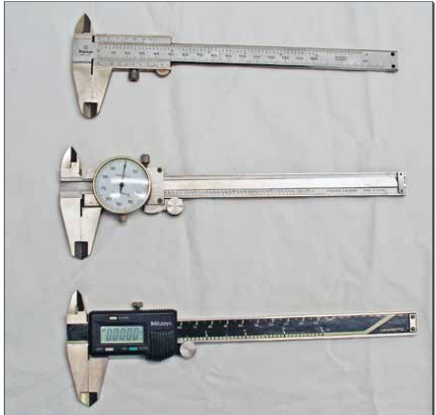
There are three main types of calipers. The vernier type (top) is usually the least expensive but most difficult to read, the dial calipers (middle) are the most common and have the advantage of not requiring a battery, and the digital (bottom) is the easiest to read but does require a battery.
