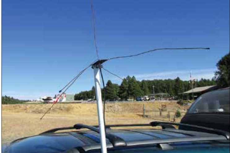
(Left) A typical airport setup for emergency communications at KGOO. The antenna is fastened to a PVC pipe and held in place by the left rear window. In the background you can see the S2 fire bomber aircraft. (Right) Close-up of the antenna. This one is around ten years old and about ready for a rebuild.
