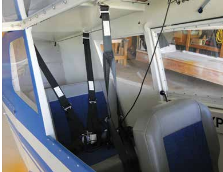
(Left) Tandem seating means plenty of elbow room. (Right) The back seat spans the full width of the fuselage, making it a great shelf for cargo when it isn't occupied by a person.
