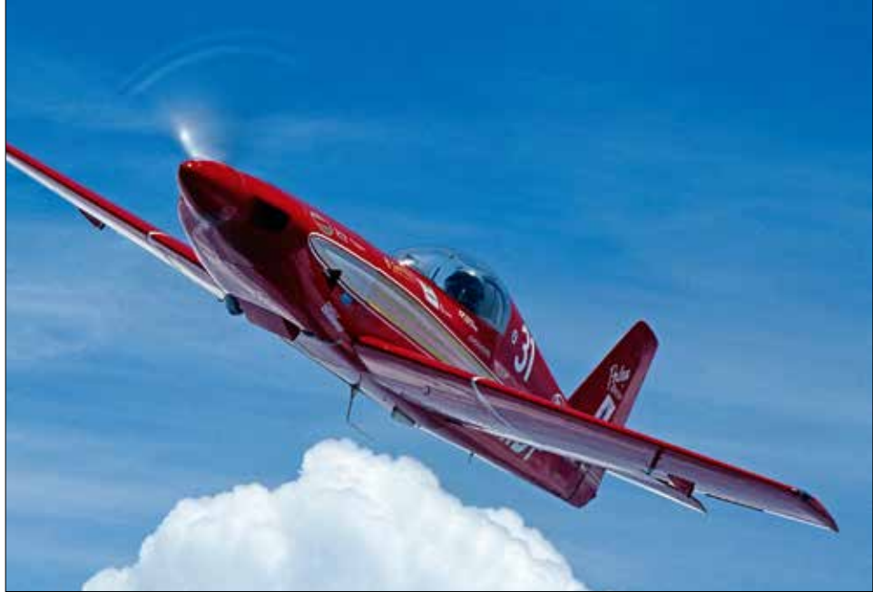
Analysis showed that adding wing fuel to the Polen Special would have lowered its flutter speed.
