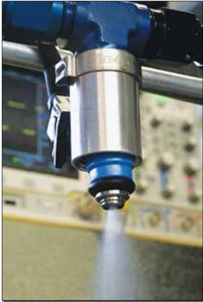
(Left) An EFII electronic fuel injector displays its well-atomized spray pattern on the EFII test bench. (Above) Both the Bendix fuel servo at left and the smaller EFII unit at right are throttle bodies. But the Bendix unit also meters fuel, hence its fuel servo name; the EFII electronic throttle body simply throttles the air supply and reports the throttle position to the computer.
