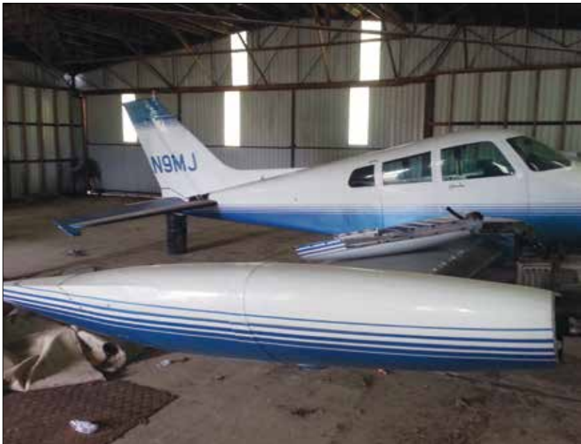
The tip tank on a Cessna 310 places the fuel well forward on the wing.
