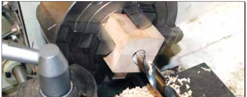
Using the four-jaw chuck, clamp the screwed-together block in the lathe, center it, and drill or bore the \frac{3}{8} -inch center hole.
