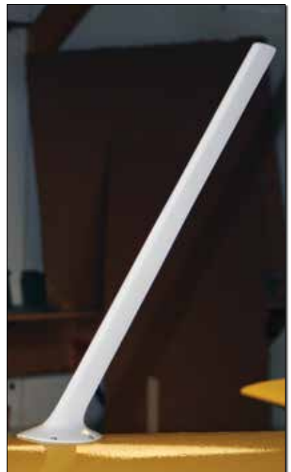
Finished antenna mounted on the RV-3.
