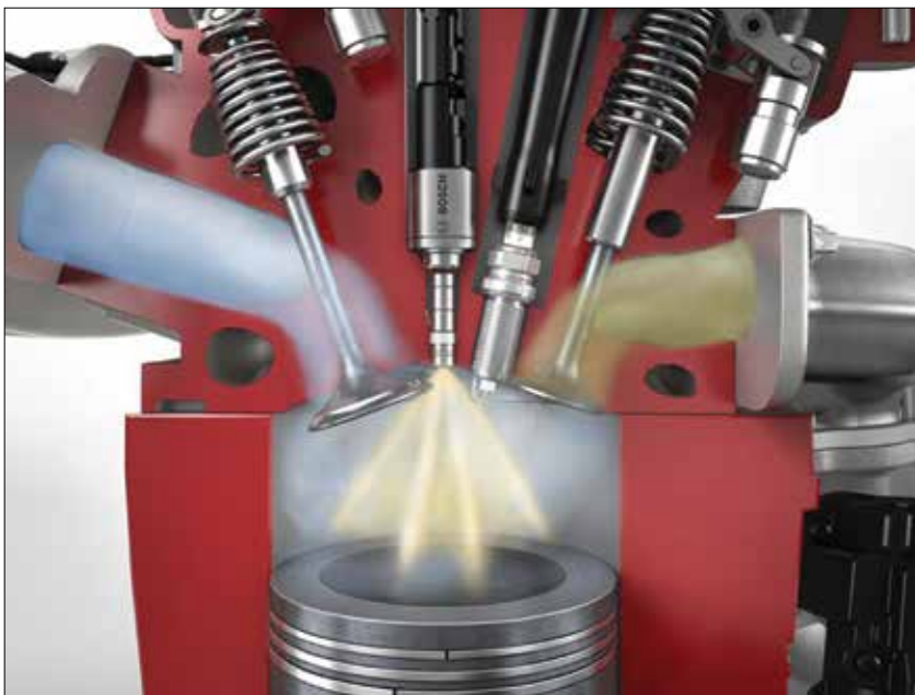
Gasoline direct injection is the new norm in automotives. Conceptually similar to diesel practice, very high pressure fuel is sprayed directly into the combustion chamber, gaining a useful quenching effect. Incorporating 2500 psi GDI to legacy aviation engines would most practically require a complete engine redesign in addition to the expensive high-pressure fuel pump and robust injectors.
