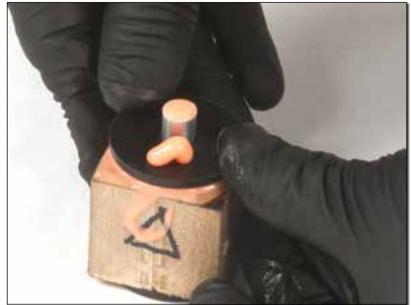
(Left) Using the manufacturer's recommended "high pour" method, fill the mold as slowly as possible. (Right) Push the cap into position and the excess will ooze out the overflow.
