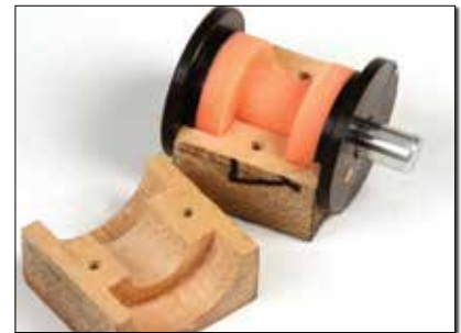
After curing at least six hours, slice off the cured rubber from the overflow and de-mold the part. As long as the mold is handled carefully, you can reuse it to make dozens of identical parts.
