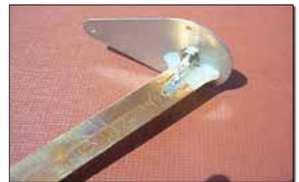
Close-up shot from 1999 shows the BNC connector soldered to the center of two 1/2-inch-wide strips of copper tape.
