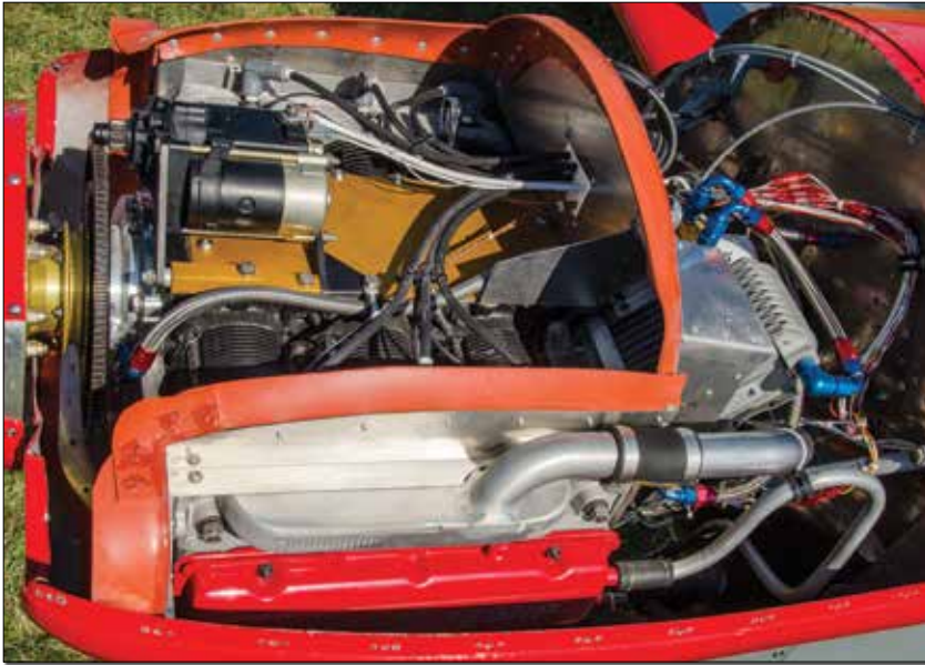
Corvair engine modified for Experimental aviation. Auto engine conversions are great options for aircraft, but they require close attention to technical details to mitigate risks and ensure reliable power. (Photo: Paul Dye)
