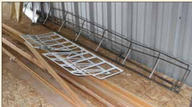
The Cassutt wing and tail kit includes these welded structures, but not much else. You'll need covering material and other items to convert these frames into usable parts. (Photo: Paul Dye)
