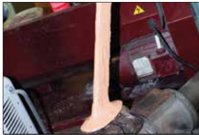
Com antenna covered with filler.
