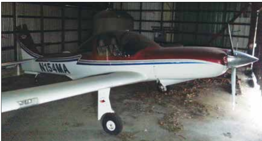
The large wing fuel tanks make this Micco SP-26 unable to meet the spin recovery requirements for an aerobatic aircraft.
