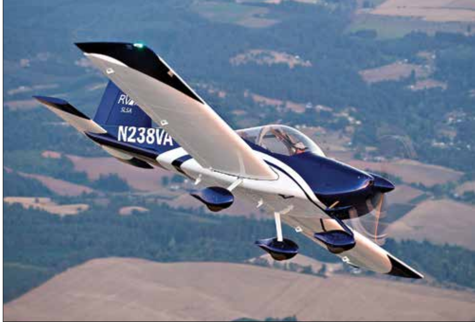
Aircraft using the Rotax 912, such as this RV-12, have fuel systems specifically designed for auto fuel.
