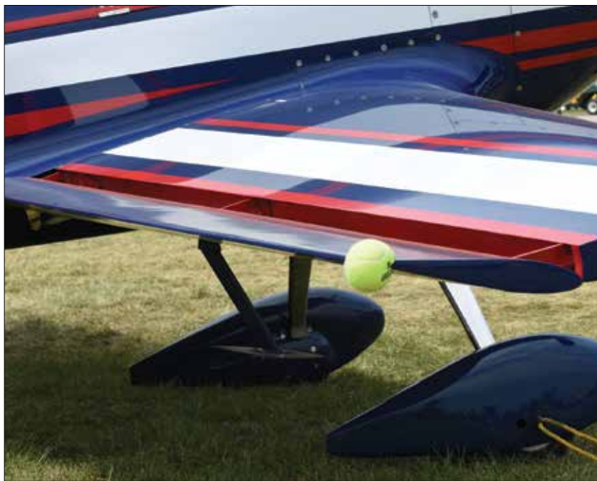
The aileron of this Giles 200 shows the set-back hinge axis and an intermediate nose shape. Note how far the aileron hinges are cantilevered aft of the wingspar.
