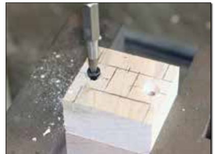
With the mold halves clamped together and the clamping holes marked, drill, countersink, and screw the two parts together as a matched pair.
