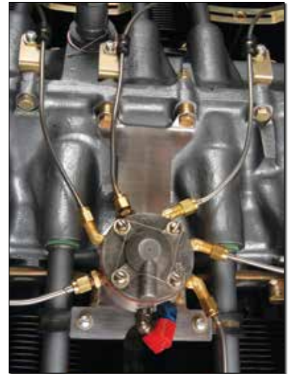
Bendix's flow divider determines fuel flow among cylinders at low fuel flow (idle, very low power settings), provides a positive flow shutoff during engine shut down, and functions as a simple distribution block at normal cruise and takeoff power settings. Under those conditions, fuel flow is determined by injector nozzle size.
