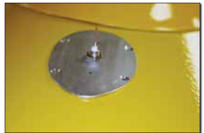
Fitting antenna base plate to fuselage.
