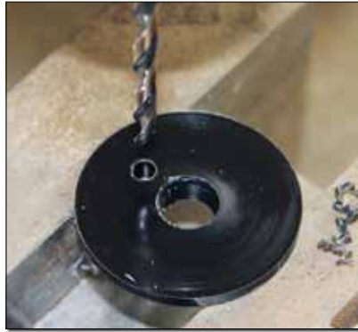
The end caps are lathe-turned from Delrin-type nylon, but any machinable plastic or aluminum will work. Drill an overflow hole into the top cap.
