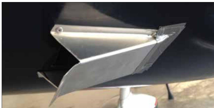
Large louvers placed over the same holes as the small louvers, but with much more projection into the slipstream.
