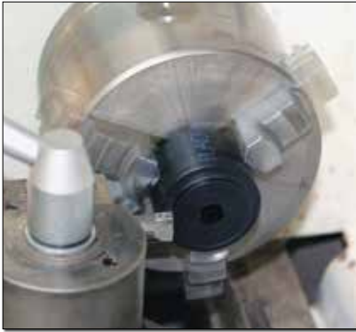
The end caps are lathe-turned from Delrin-type nylon, but any machinable plastic or aluminum will work. Drill an overflow hole into the top cap.
