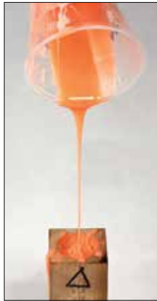
(Left) Using the manufacturer's recommended "high pour" method, fill the mold as slowly as possible. (Right) Push the cap into position and the excess will ooze out the overflow.
