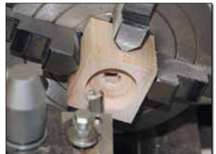
Using the boring tool, face the block flat and counterbore the flange cavity. Flip the block and repeat the facing and counterbore operations on the opposite side. When done, remove any stray wood fibers with 180-grit sandpaper. A coat of acrylic clear coat and some mold release wax will seal the wood and prevent the rubber from sticking.
