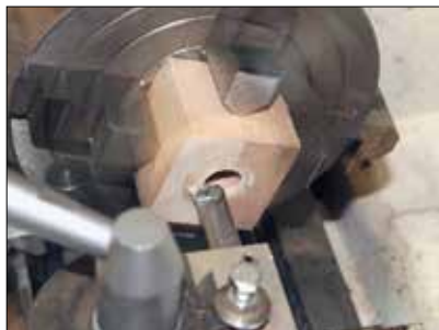
Using the boring tool, face the block flat and counterbore the flange cavity. Flip the block and repeat the facing and counterbore operations on the opposite side. When done, remove any stray wood fibers with 180-grit sandpaper. A coat of acrylic clear coat and some mold release wax will seal the wood and prevent the rubber from sticking.
