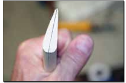
Top view of antenna shows its airfoil shape.
