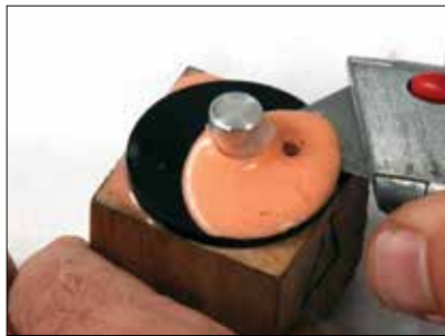
After curing at least six hours, slice off the cured rubber from the overflow and de-mold the part. As long as the mold is handled carefully, you can reuse it to make dozens of identical parts.
