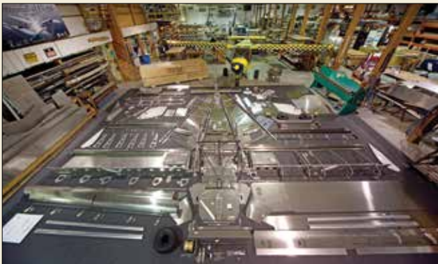
The kit for the Zenith STOL CH 750 includes virtually everything you need to build the airframe. (Photo: Courtesy of Zenith Aircraft Company)
