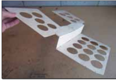
In contrast, the forward backing frame is a more complex shape due to the wingspar that passes below the pilot's legs. A frame is especially helpful in cases like this where the cushion is not sitting flat. Lightening holes optional.
