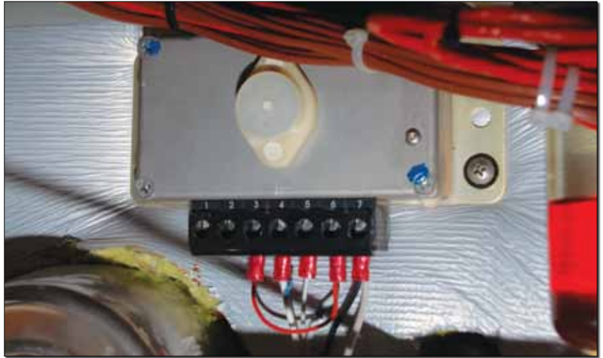
This airplane uses a B&C solid state voltage regulator. It will work better if it is installed inside the cabin instead of in the engine compartment. One advantage of the B&C regulator is that the voltage is easily adjustable.
