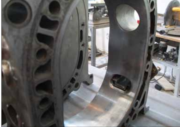
A peripheral intake above and slightly modified exhaust port below. Peripheral ports almost double the horsepower at the expense of a rough idle.
