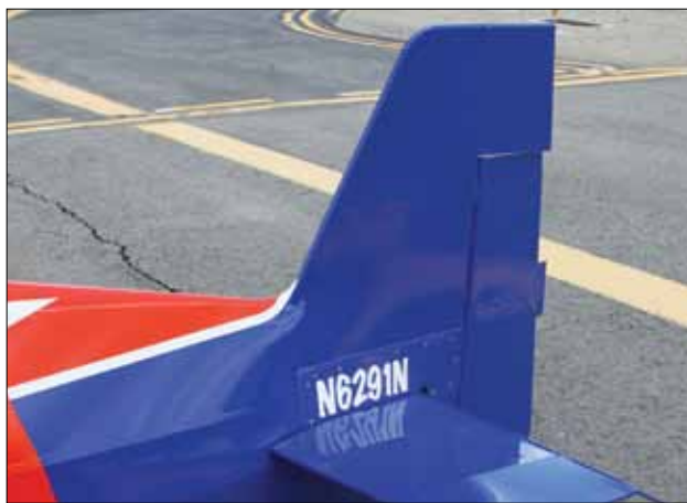
King's aircraft has a slightly taller vertical fin than called for in the plans for added stability. Pitch trim is accomplished by adding or subtracting washers on the stabilizer attach points.
