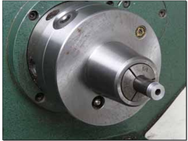
A 5C collet system mounted to the lathe. This particular model uses a scroll system with a T-handle to tighten the collet.
