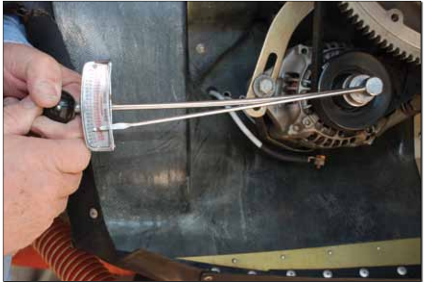
Be sure to check the tightness of your alternator belt yearly and whenever you are having alternator problems.
