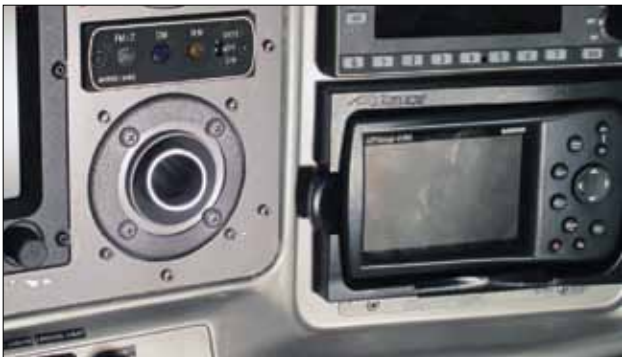
The system includes three cabin heat outlets. Two were installed near the floor on the pilot and passenger side, and one installed in the instrument panel.
