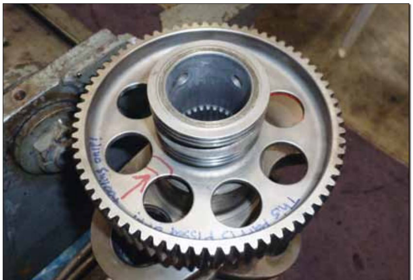
See the crack in that gear? Many would have missed it. Careful inspection is a good lesson homebuilders can learn from the racing crowd.
