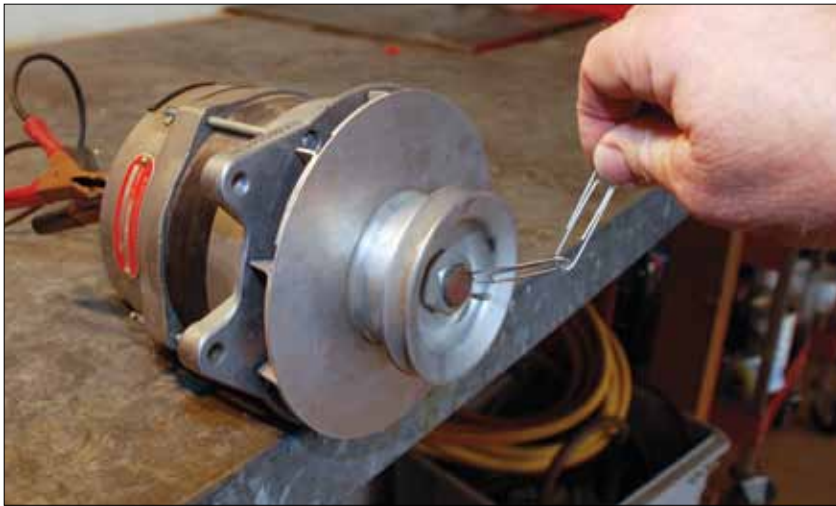
A quick test to see if the field is working is to power up the field and see if the rotor shaft is strongly magnetized. A tester made up of two paper clips shows that it is.
