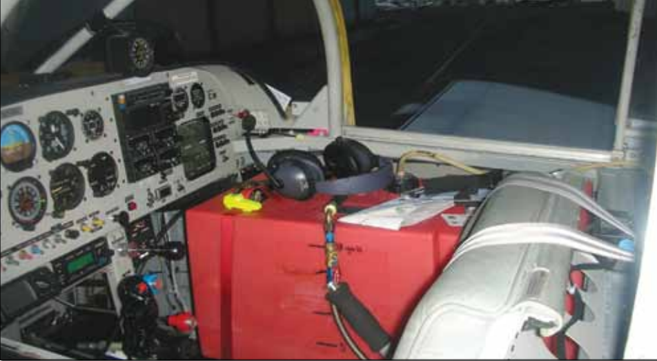
View of cockpit showing the auxiliary fuel tanks that allowed an extra six hours of flight.
