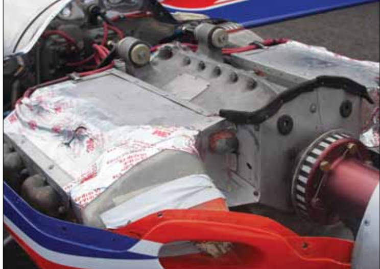
The firewall-forward design is simple and uses individual plenums for cylinder-head cooling.
