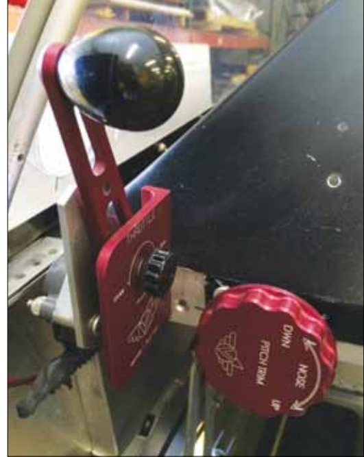
Even if you're building from plans, there are some parts that just aren't worth the trouble to make from scratch. This throttle and trim control are good examples.
