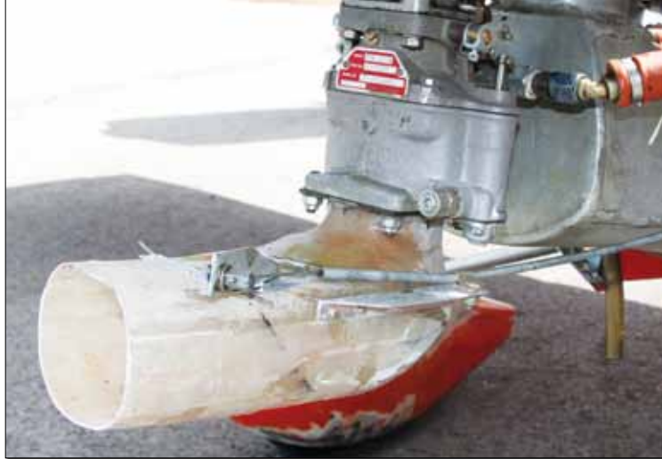
King added a cylindrical carb air inlet during his rebuild project to replace the former boxy-looking rectangular scoop. The fiberglass air box matches the round inlet snout. Note the custom-made oil tank, shaped to fit in the compact Cassutt cowling.
