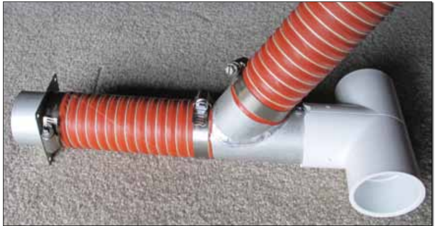
Cabin heat plenum. A 90° elbow (not shown) attaches to the 2-inch flange duct and keeps the plenum away from rudder pedal movement and brake lines.
