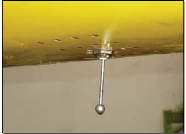
How much faster could Voodoo go with a low-drag transponder antenna? We don't know—but we'd like credit for the idea if they change it and go faster!
