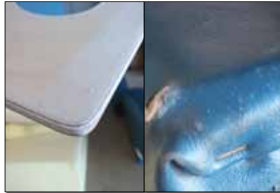
Corners should be rounded and edges radiused to minimize possibility of frame rubbing through upholstery.
