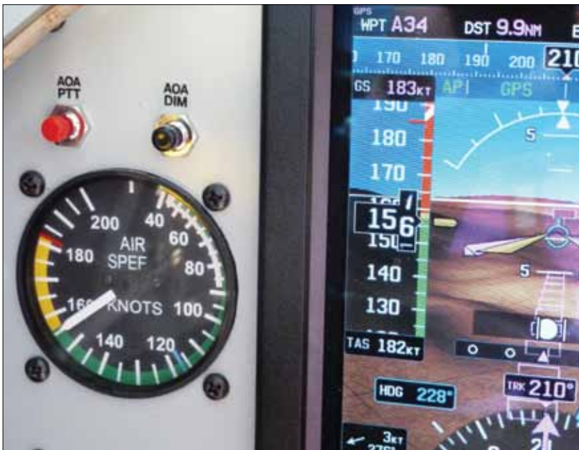
Most modern EFIS displays can adjust the redline to represent the current IAS that corresponds to a fixed TAS redline. This often makes the yellow arc (or band) become very small or disappear completely on the airspeed indicator, as is evidenced in this high-flying picture.
