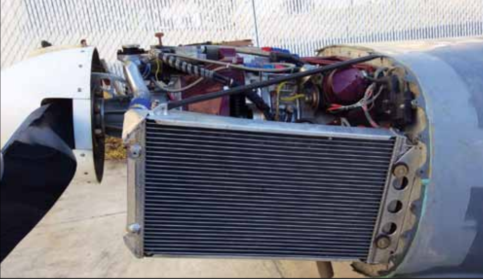
Fourth radiator; third oil cooler, engine mount, and overhaul; second oil tank, ignition, gear reduction, rotor, bearings, etc. This is the final iteration, the author hopes!
