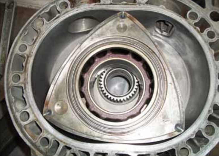
The rotor comfortably nestled in its toroidal chamber. No valves, lifters, cams or timing chains. In theory, fewer parts means less chance of failure.
