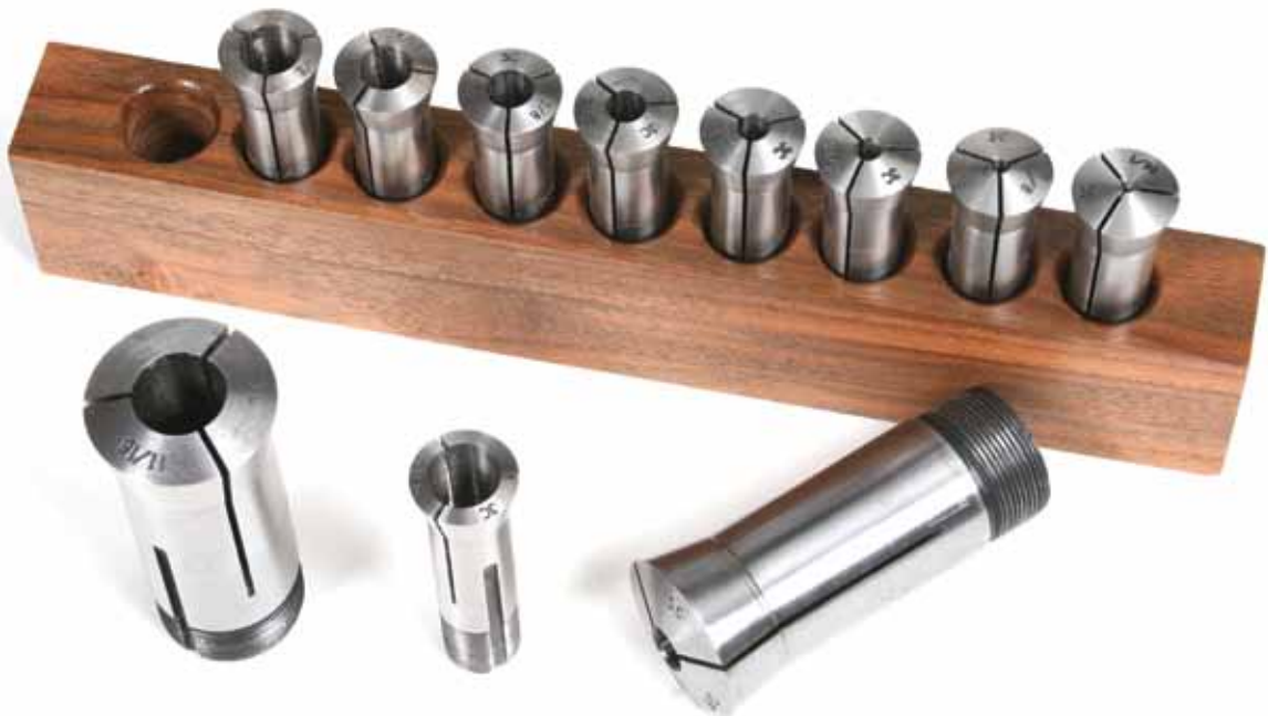
This comparison shows the relative size difference between the "standard" 5C collets and the mini-lathe 3C collets. Collets are precision tools that should be stored in an appropriate tool holder.
