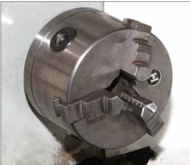
L: A typical three-jaw self-centering chuck. R: Independent jaw chucks hold odd shapes.
