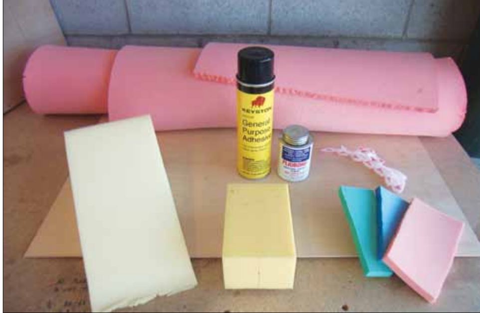
Materials for DIY seat. Foam (L to R): Medium-density "rubberized" urethane foam, high-density "tractor" foam, and high-, medium-, and low-density CONFOR foam. Large roll of pink CONFOR foam in the back. Foam-compatible spray adhesive, as well as brushable Pliobond for touchups. Velcro may be necessary to hold cushions in place on some planes. Materials are resting on a sheet of 3mm birch ply used as a backing frame.
