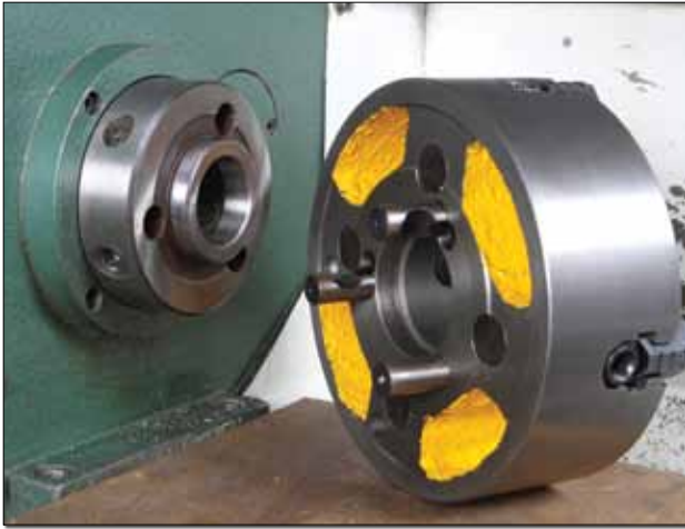
The D1-4 cam-lock system: three studs in the back of the chuck mate with the spindle. A 90° turn on each of the three cams secures the chuck.
