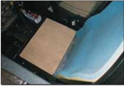
The simple rectangular rear bottom seat cushion backing frame is checked for fit. Seat back has already been completed in this photo.
