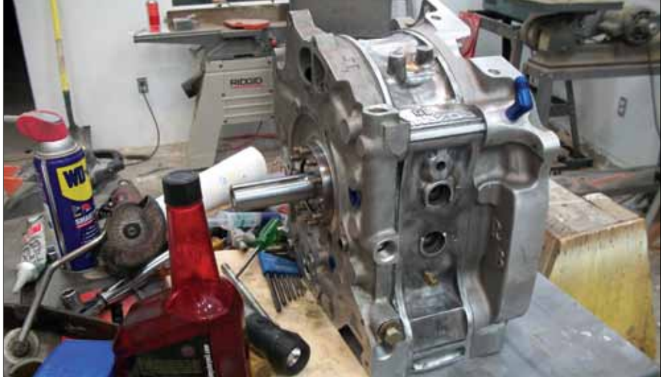
The assembled block weighs 68 pounds, about the size of a large battery. Not bad for 140 horsepower.
