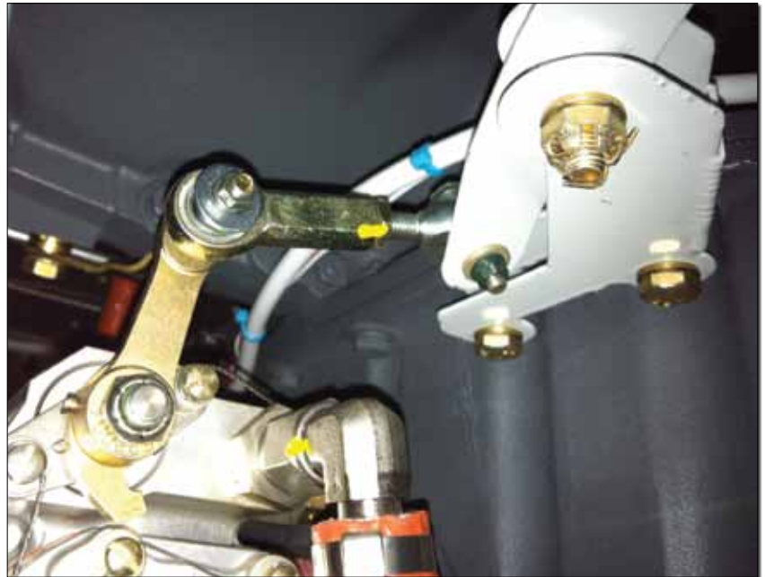
Here's a great example covering a number of things: Torque Seal on B-nuts and jam nuts, cotter keys on bolts subject to rotation, and metal lock nuts in the engine compartment.
