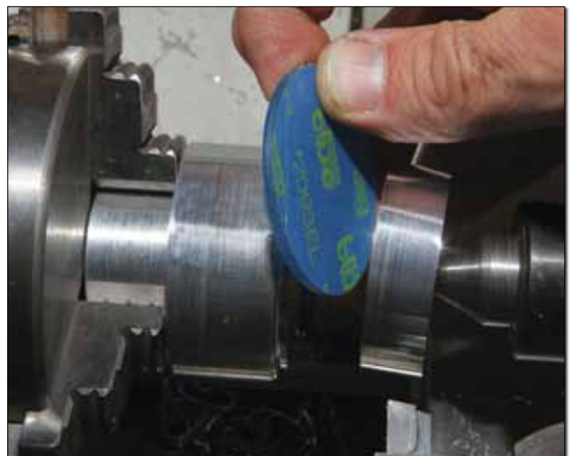
In this variation of between centers turning, a small sheet of Plexiglas is turned to a perfect disk (the tape is to prevent scratches). This method can be used to turn any material that is too thin or fragile to machine any other way.
