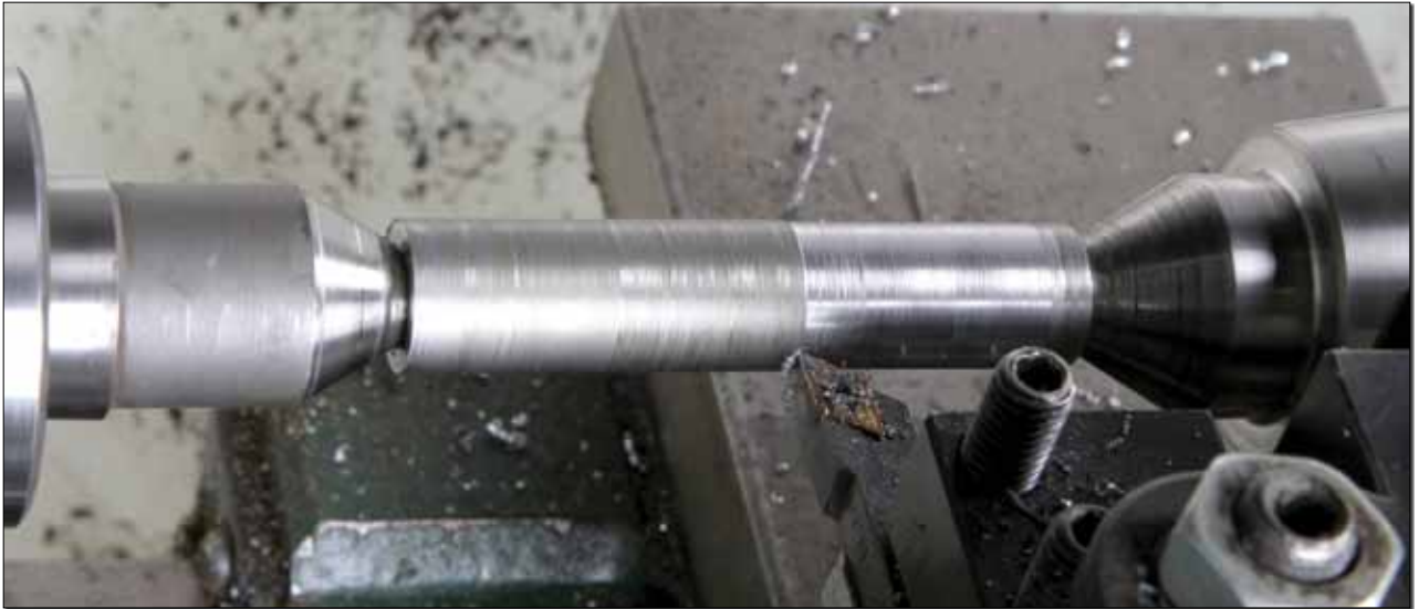
The clamping force of the tailstock live center (right) is often enough to engage the drive center for taking light cuts.
