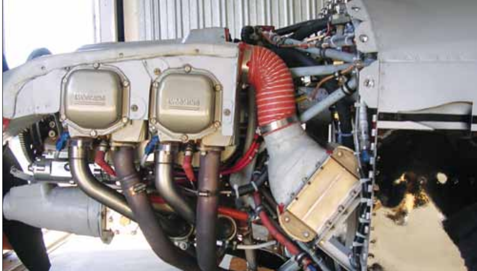
Engine detail showing IO-360 with cooling air plenum, electronic ignition, and ram-air horizontal intake.
