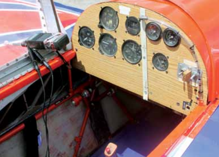
The simple cockpit has only two switches—one for the left mag, and one for the right. Basic instruments include a sight gauge for the fuel tank.
