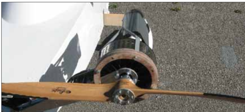
Without streamlined cowling, Electravia's record-holding Cri-Cri shows close connections between motor, controller. Note longer lines going to batteries inside fuselage.
