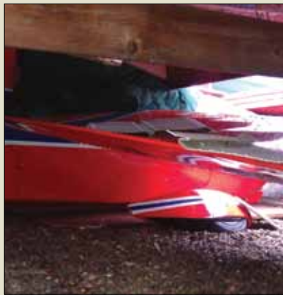
The landing gear was smashed flat, and the wheelpants damaged—but the primary structure was in good shape.
