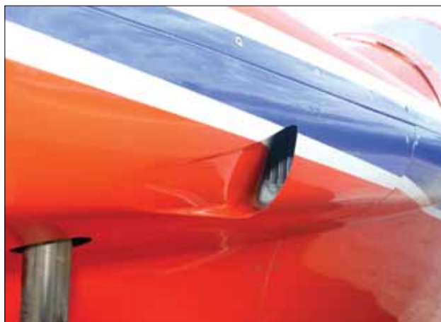
Oil cooler air comes from a scoop on the right side that is sculpted to provide better flow at slow speeds/high angles of attack. The outlet is above the wing at the root.
