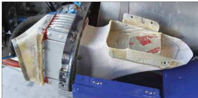
The oil cooler installation on King’s airplane is so effective that he has to partially block it off in order to get temperatures up to operating values.
