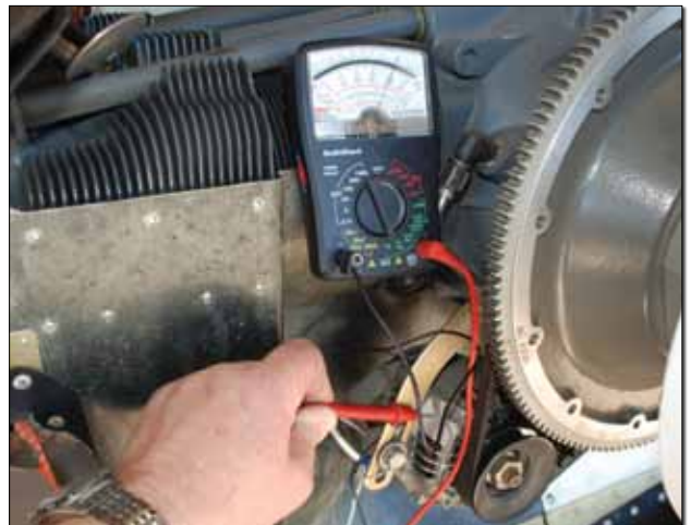
When testing an alternator with only an F terminal, one lead goes to the case (ground) and the other to the F terminal. This B&C alternator shows 5 ohms field resistance, which is exactly right.
