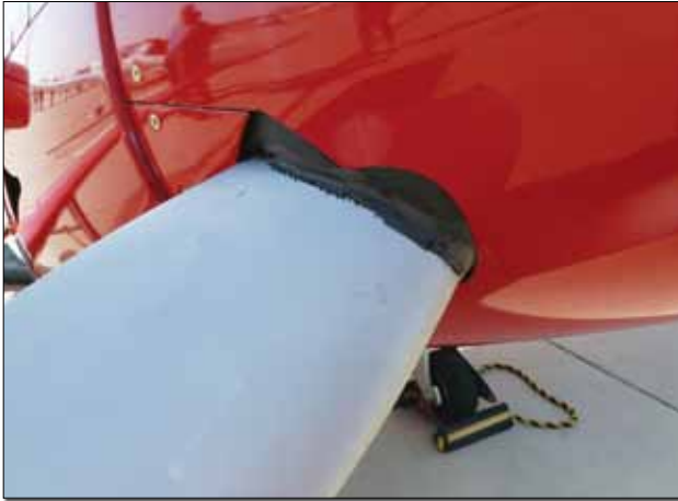
How much speed is gained by adding these seals to the prop/spinner gap on this go-fast machine in Mojave? The owner wasn't saying—but you can bet he knows!
