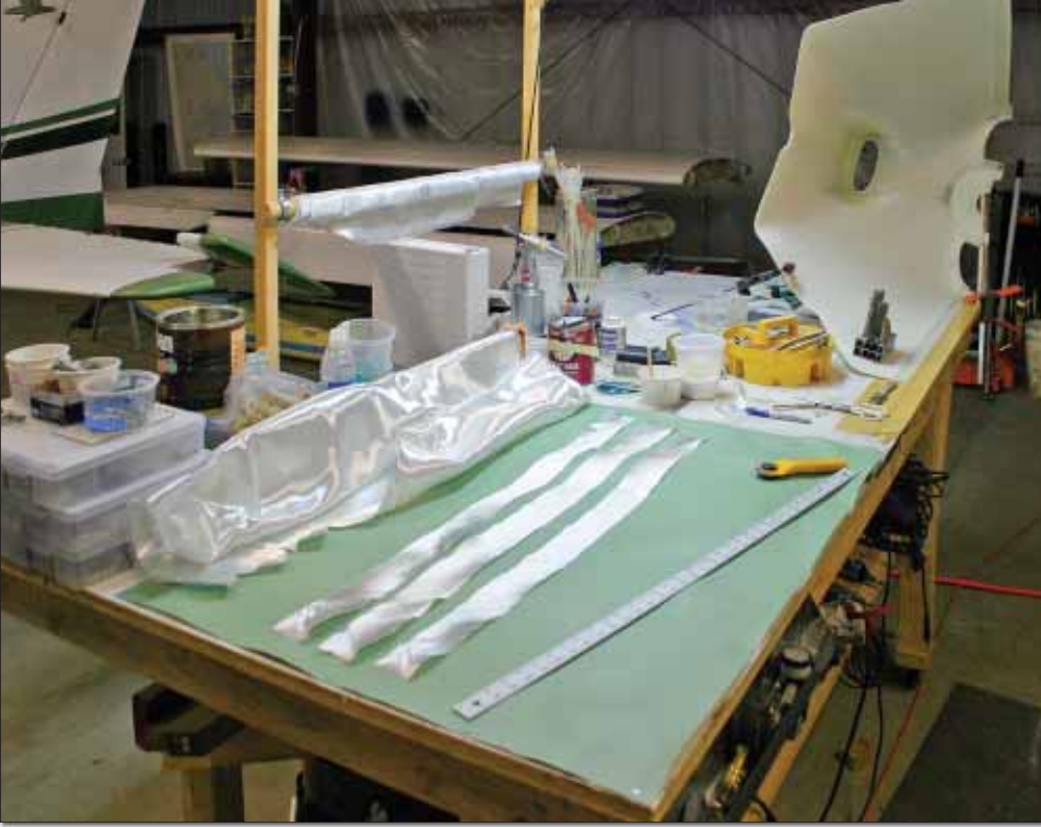
Brown packing tape on the table, cowl in position, glass is cut and ready for application.
