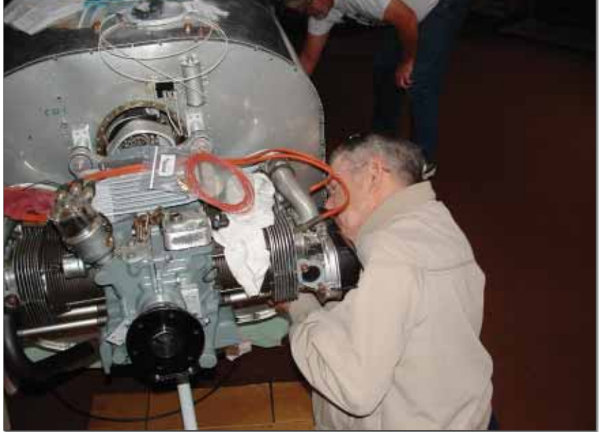
Mel Ellis drills the VW sump for installation of an oil temperature sender. Hint: Grease on the bit captures drill chips.
