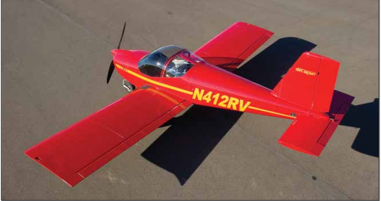
The Van's RV-12 is unusual in light Experimental aircraft for use of a stabilator—the all-flying horizontal tail. Choosing the proper hinge line for this configuration is critical. Randy Schlitter's RANS S-19 LSA also uses a stabilator.
