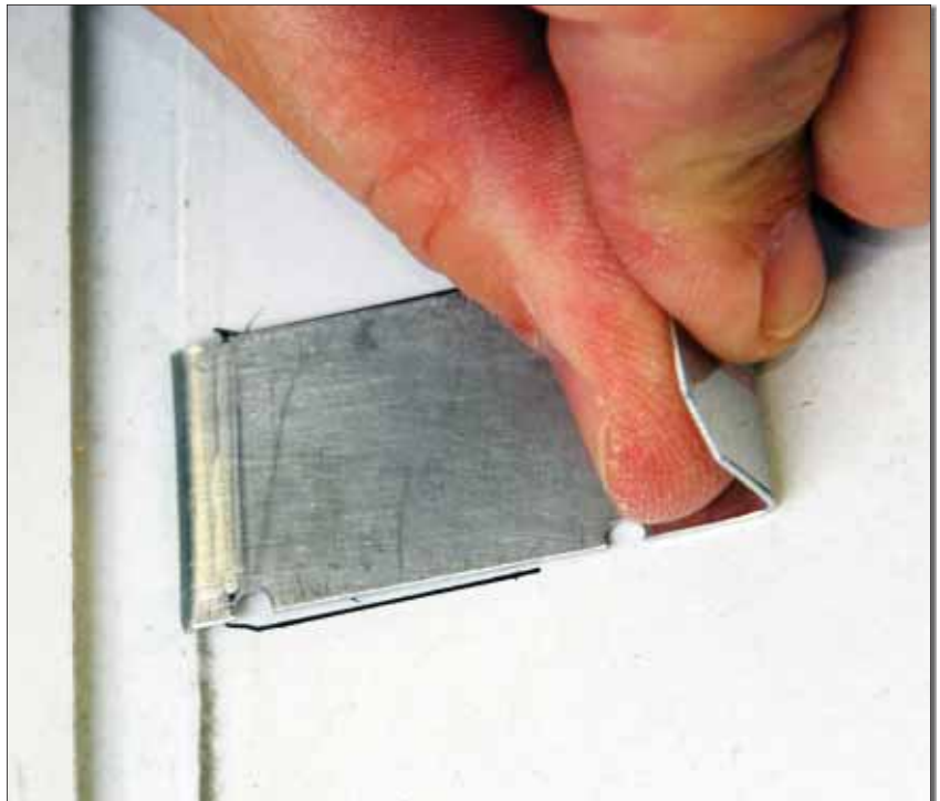
This simple improvised aluminum tool hooks onto the fuselage joggle.
