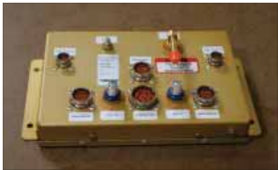
The heart of the Eagle EMS is this ECU module, which is intended to be mounted on the hot side of the firewall.
