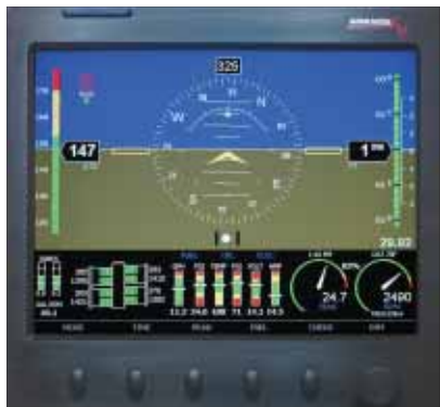
Advanced Flight's engine monitor can be displayed on an EFIS screen (left). A weight-and-balance screen helps loading (right).
