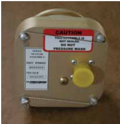
Each magneto pad is populated by a speed sensor. This is the back side (left) and the engine side, less the drive gear (right).
