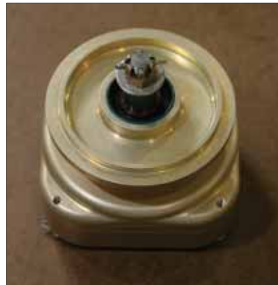
Each magneto pad is populated by a speed sensor. This is the back side (left) and the engine side, less the drive gear (right).
