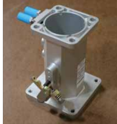
A simplified throttle body has pickoffs for induction air temperature and manifold pressure.
