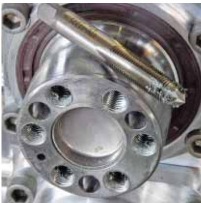
One threaded hole cleaned, five to go.
