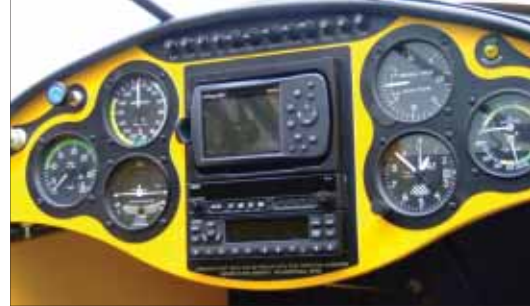
A Garmin GPS receiver has been added to this standard-equipment panel.
