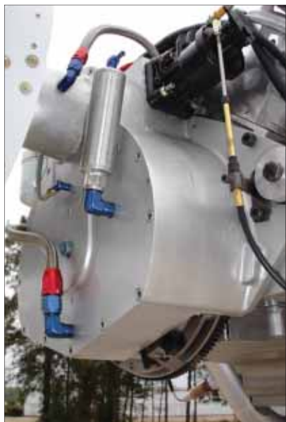
Geared Drives PSRU.
