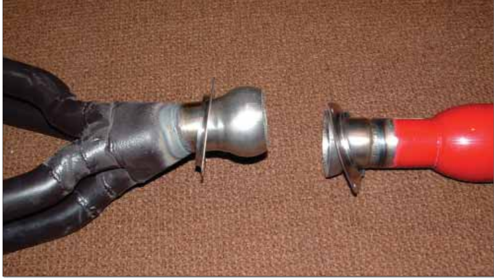
The four-into-one exhaust is coupled to an aftermarket auto muffler. Heavy, but the result is an extremely quiet airplane.
