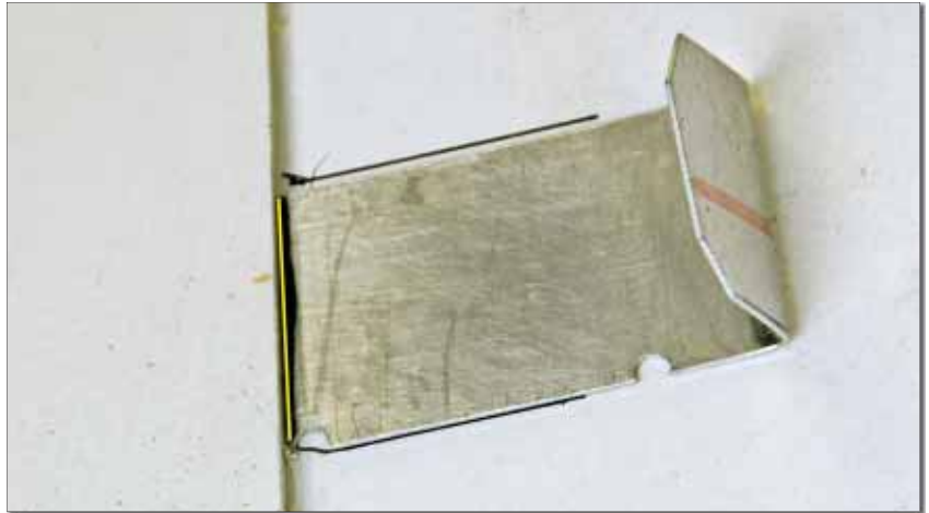
Hook the tool on the joggle, and then mark (yellow/black line) the overlap on the tool with a Sharpie.
