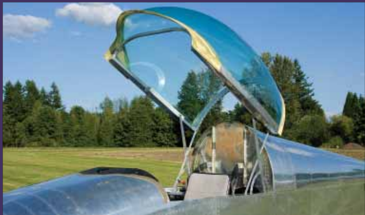
The scissor-action lifting canopy solves many problems, but it demands careful operation.
