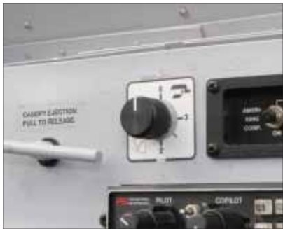
This knob is the pilot's only onboard control of the fuel/air mixture.
