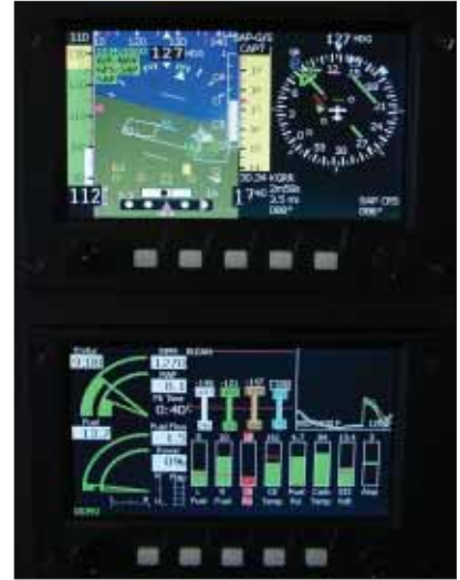
Interactivity is important. The Grand Rapids models can be connected to share engine information with the EFIS.
