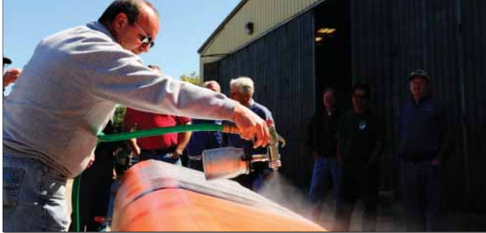
Spraying with a high volume low pressure (HVLP) system such as the one shown here reduces the amount of overspray.
