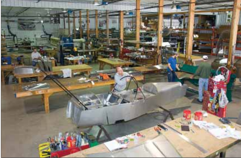
In the Zenith shop, quickbuild components for the CH 600 line are assembled. While plansbuilders can still build any Zenith the traditional way, the business has definitely swung toward more work from the factory.
