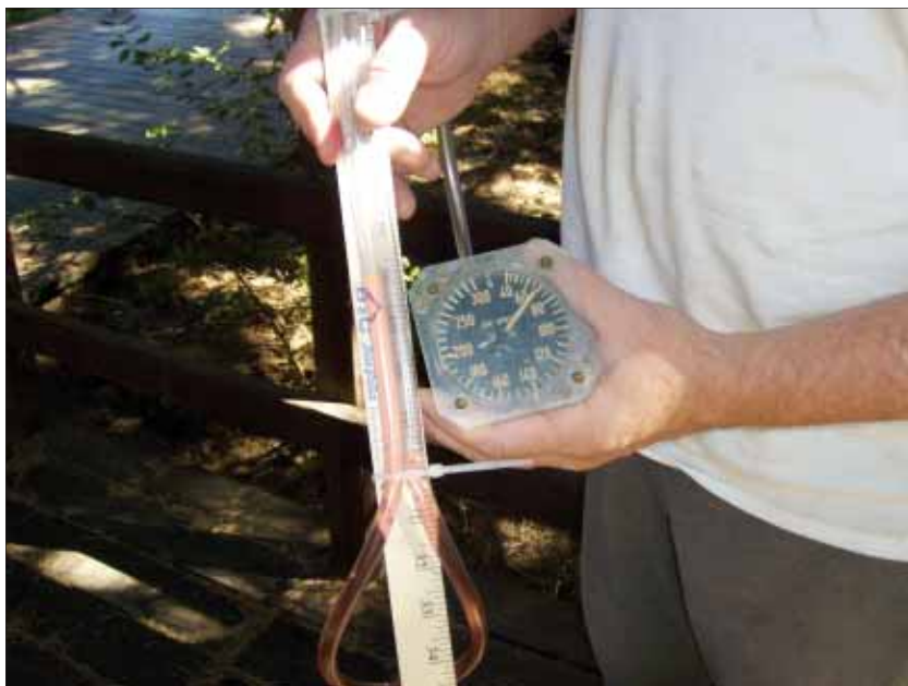
Calibration at 70 mph indicated airspeed is right on (factoring in the fact that this photo was taken at a density altitude of 3000 feet MSL).
