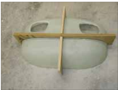
The nose bowl mold, pulled from the plug and reinforced.
