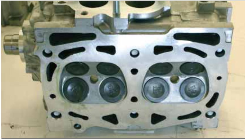
Subaru's single-overhead-cam, four-valve-per-cylinder head is tuned for good torque production.
