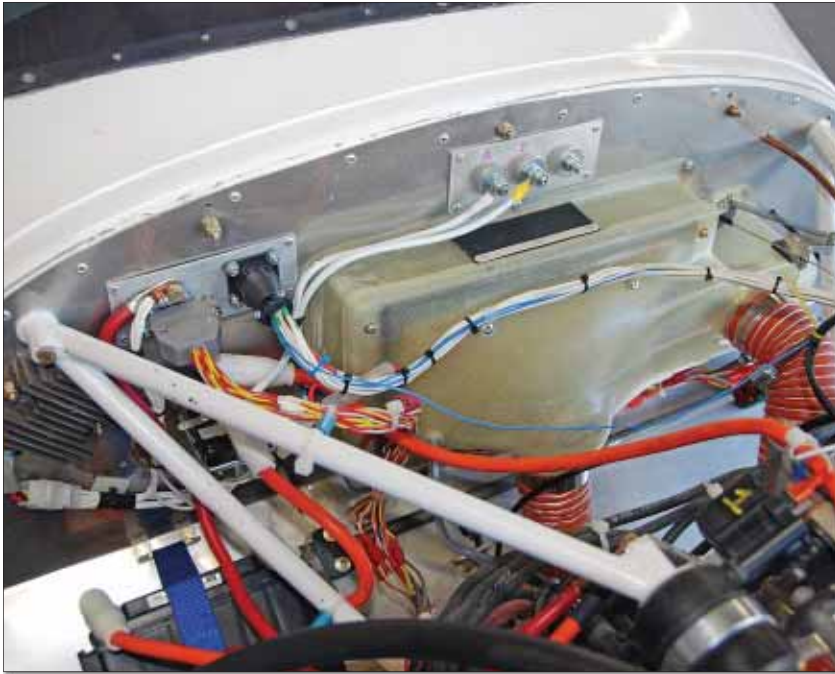
On the left is the voltage regulator; the airbox is in the middle. You can see why it's important to mount at least the airbox before you hang the engine.
