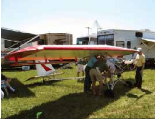
With a whole crowd of interested heads in the way, watching, the insertion and tightening of the four wing attach bolts took a little longer.
