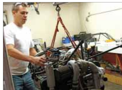
Craig Woolman wheels the prototype turbocharged EJ25 into the Maxwell dyno cell. Testing is ongoing for the 195- and 240-hp versions.
