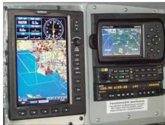
Size matters: Installed in this GlaStar Sportsman's panel next to a 496 in an Air Gizmos mount, the 696's much larger form is plain to see.
