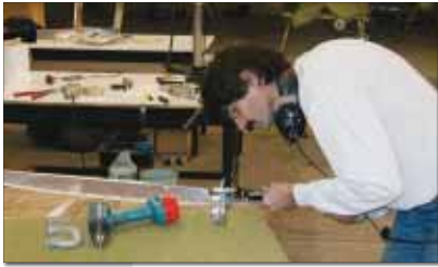
How many airplane designers get to actually build what they design? Krueger squeezes rivets.
