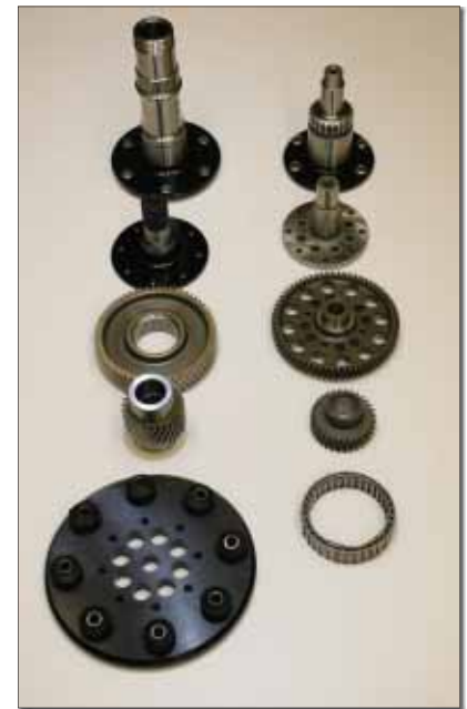
The Maxwell PSRU internals are stacked on the left, and the previous NSI major components are on the right.
