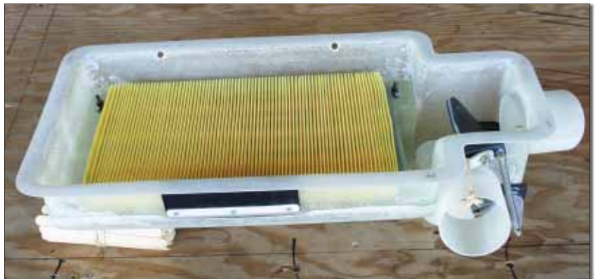
The air intake box before mounting. It contains an easily replaced filter.
