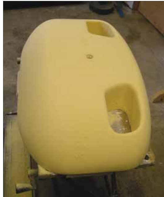
The nose bowl plug nearing completion. The author's long dormant surfboard-shaping skills came back surprisingly well!
