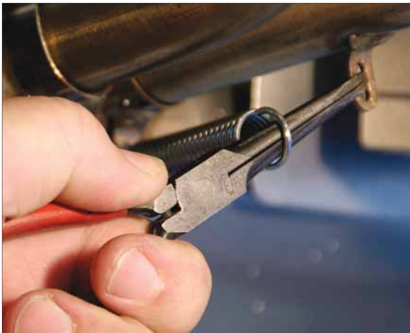
Levering the spring onto the ring this way will avoid putting any nicks in the spring wire.
