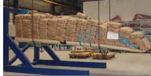
For testing positive-G capability, the wing is inverted and loaded according to a distribution plan.
