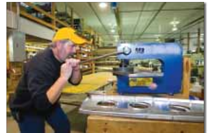
Zenith kits are well-known for their simplicity, and even at the factory processes such as flanging wingrib lightening holes are performed the simplest way possible.
