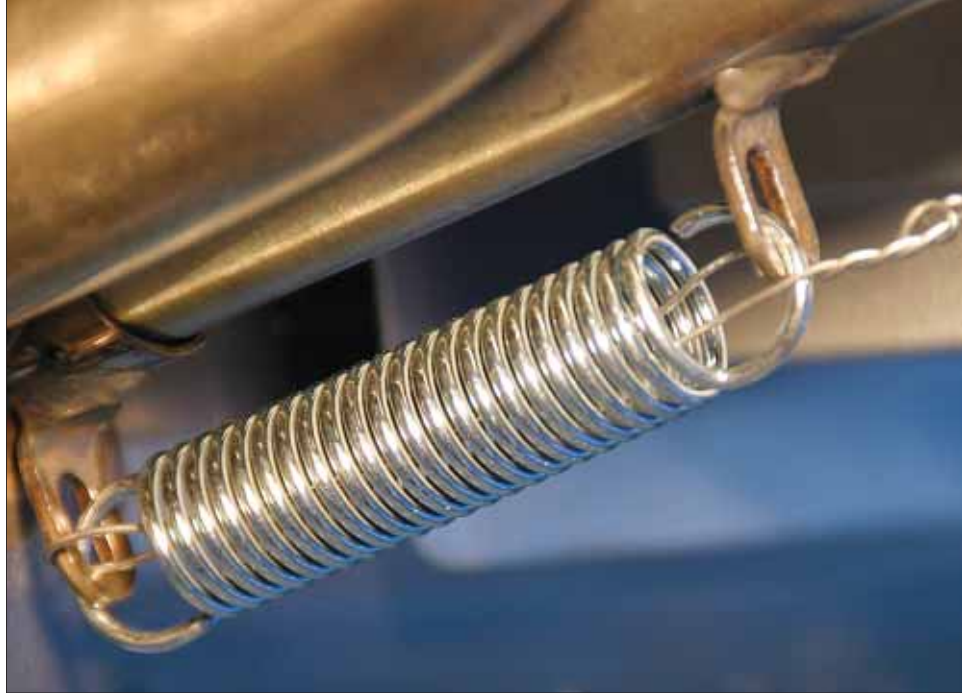
The safety wire through the middle will keep the pieces together if the spring breaks.
