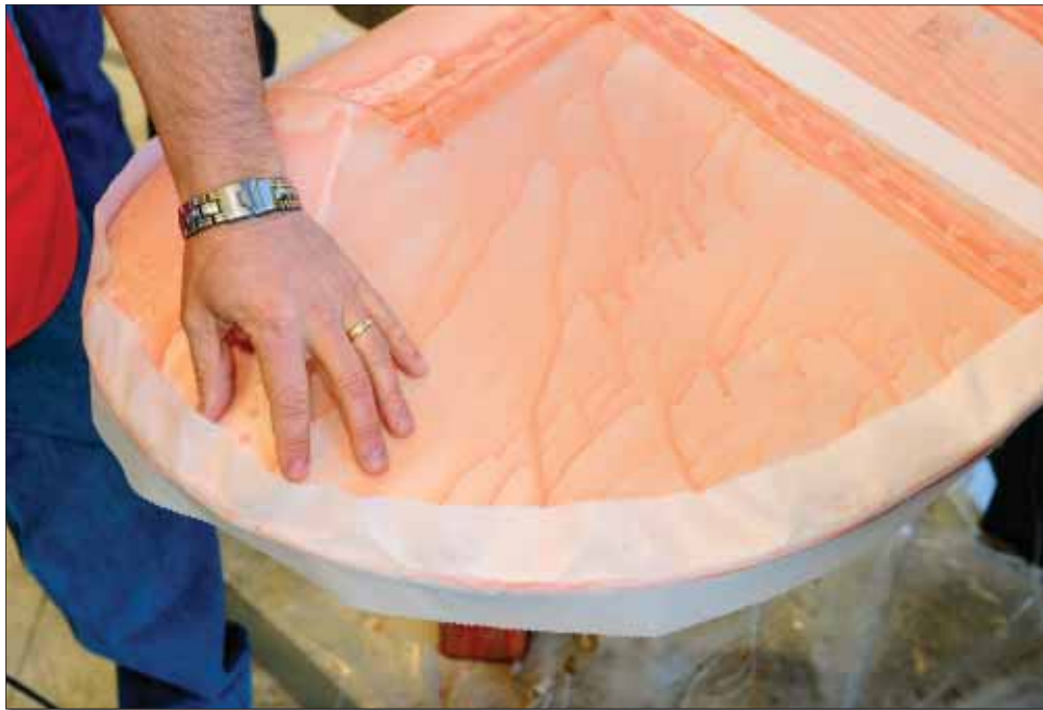
You can work a straight tape around a curved area as shown. The advantage of a linear or straight tape, as opposed to a bias-cut tape, is that there are no seams to deal with during the application.
