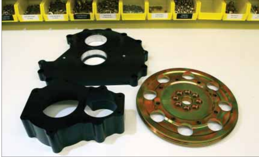
Maxwell completely redesigned the PSRU carrier from a cast piece to a fully machined and black-anodized aluminum part. Gold flywheel (right) is the starter ring gear (minus teeth) and receiver for the rubber-isolated transfer plate.
