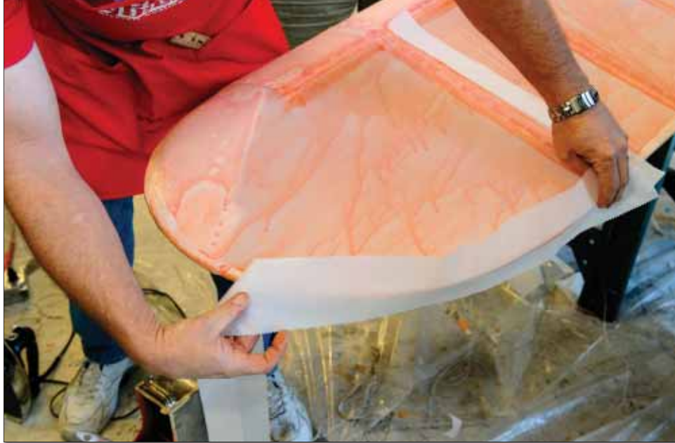
Begin taping a curved area by securing the tape at one end. Be sure to cut the tape to the proper length before applying.
