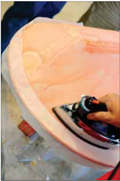
All of the wrinkles that may occur in the tape can be worked out of the fabric by using the heat from an iron to smooth and form the material.
