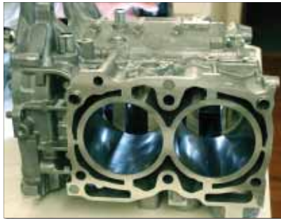
By using a WRX STi turbocharged block, Maxwell bolsters the conversion's bottom-end strength and paves the way for a turbocharged upgrade later.
