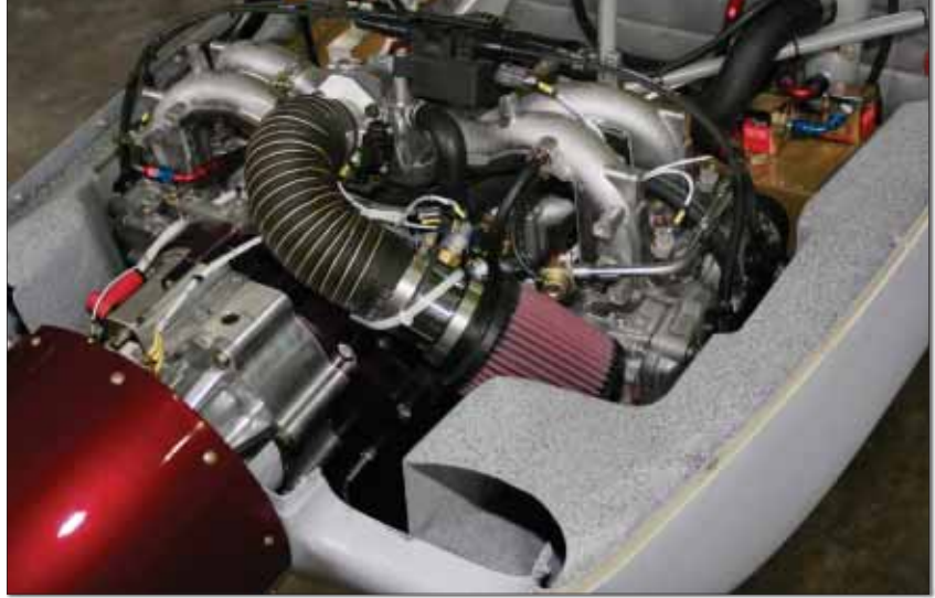
Ducts outboard of the cylinder heads feed the firewall-mounted radiator. The Maxwell conversion retains the Subaru's mass-airflow sensor, visible on the pipe between the K&N air filter and the SCEET hose to the throttle body.
