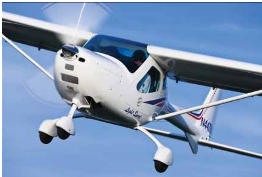
The Remos GX features an all-composite wing designed for 4 G and ground-tested to 8 G.
