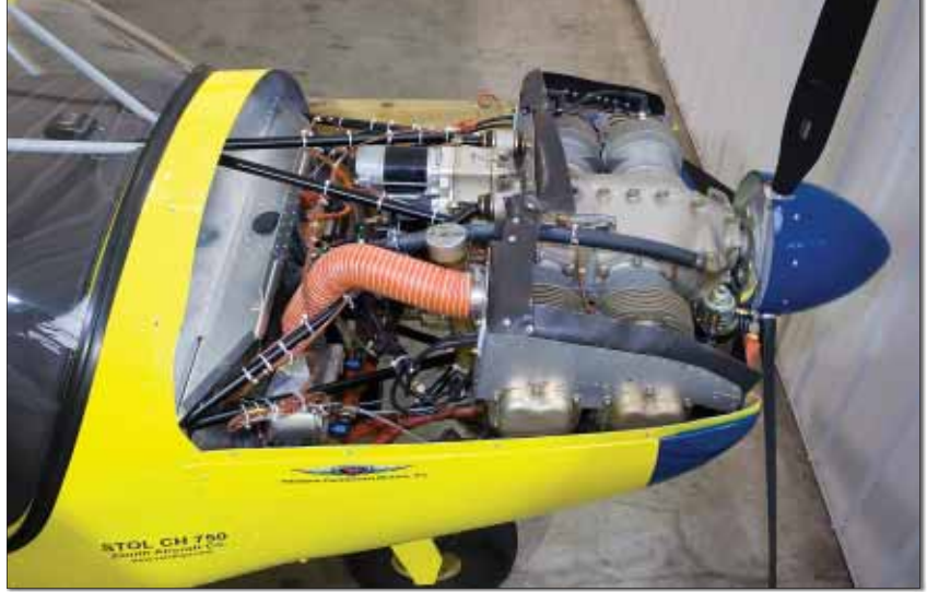
Zenith fitted the venerable Continental O-200-A (100 horsepower) to the factory CH 750, but the airframe will handle engines of 80 to 120 hp, up to 300 pounds installed weight.
