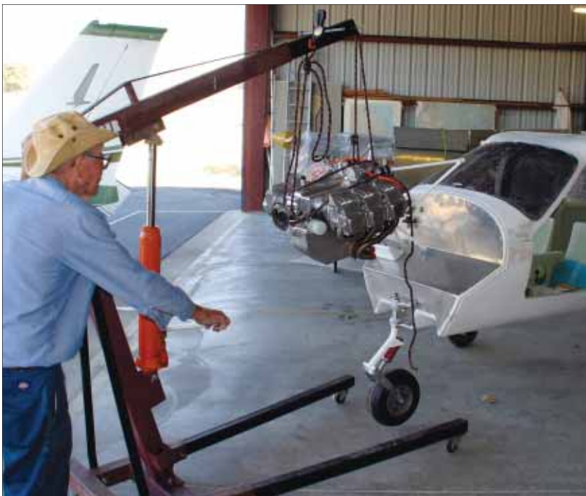
The author's friend Buzz brought his engine hoist over to make short work of positioning the engine with the mount attached.
