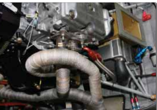
The compact Subaru engine exhales through a near-equal-length tubular exhaust, wrapped to keep the cowling cool.
