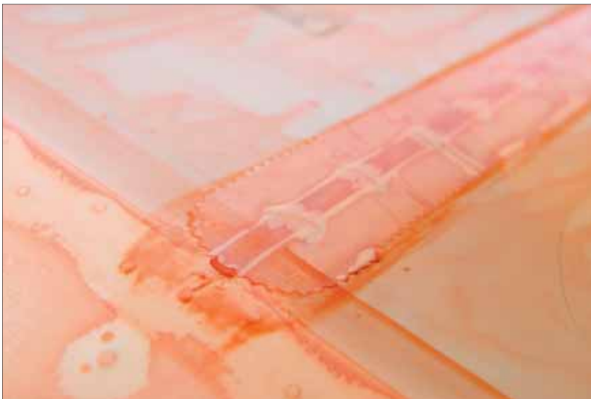
Tapes may be cut so that they are rounded on one end to make for a more pleasing finished appearance.
