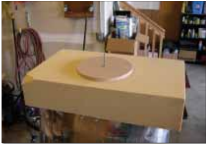
Starting the nose bowl plug. The disk represents the diameter of the spinner.
