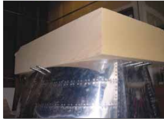
The front of the all-metal cowl determines the shape at the back of the nose bowl.
