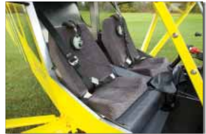
Two seats with room to spare. Nominal cabin width is 42 inches, but that can be expanded by a massive 8 inches with optional bubble doors.
