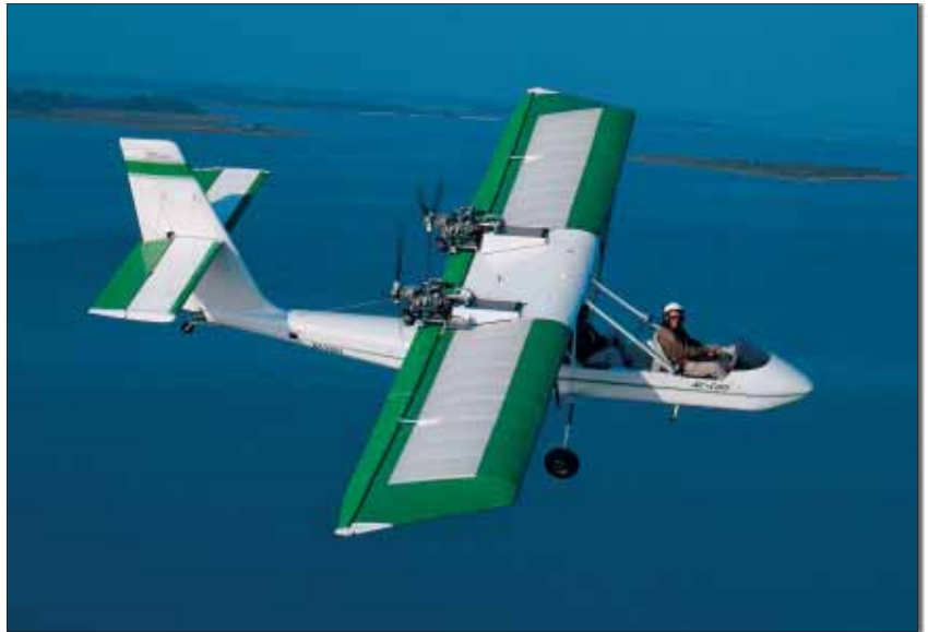
The AirCam, among the very few multi-engine Experimentals, has excellent single-engine handling characteristics in part because the engines are laterally close together.
