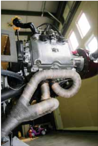
Compact and respectably light, the EJ25, as used in the Maxwell conversion, produces 165 horsepower.
