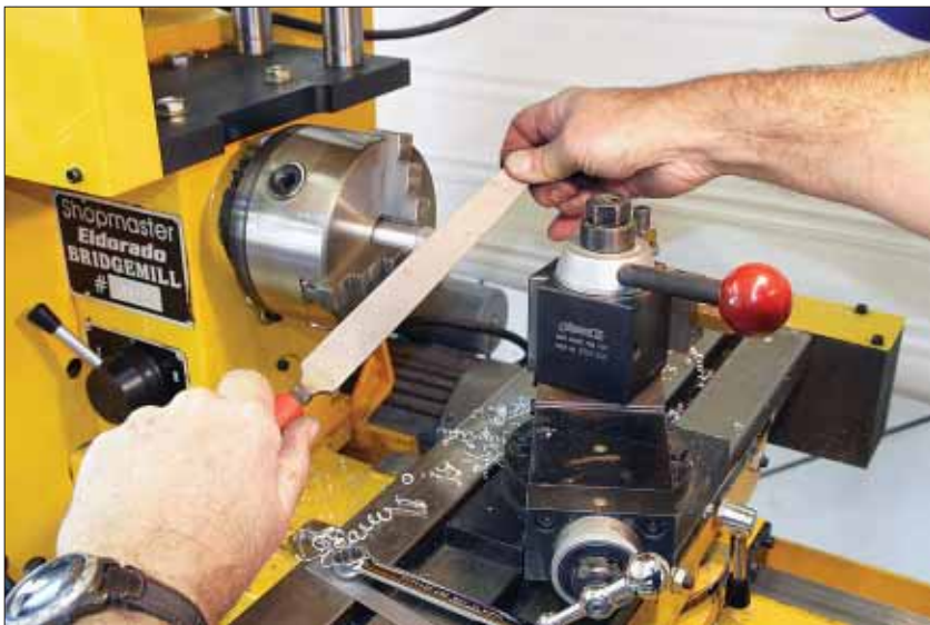
Although you could cut the chamfer, a file does a dandy job. Note that the author is in short sleeves and is working without going over the rotating chuck.
