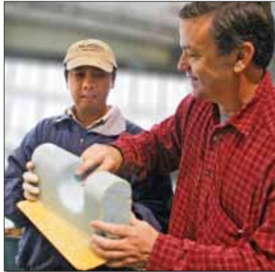
The sides are flat, and, ignoring the saddle at which Mark Wainwright is pointing, the curve over the top means a rectangular shape of material will cover it all.
