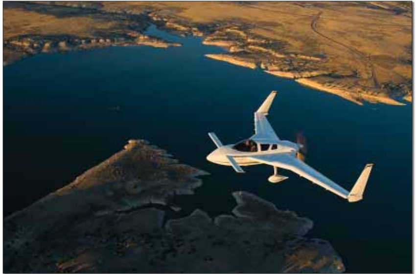
Transoceanic it's not, but the Cozy has solid cruise performance. It needs long runways, relatively speaking, but has great crosswind capability in the right hands.
