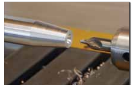
Center drilling removes any vestige of a high spot. This makes the subsequent drill bit find exact center.
