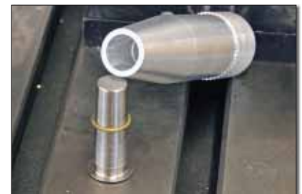
Place the large half of the tool onto the taper, push the steel ring down the taper, and snap it on to the receiver.
