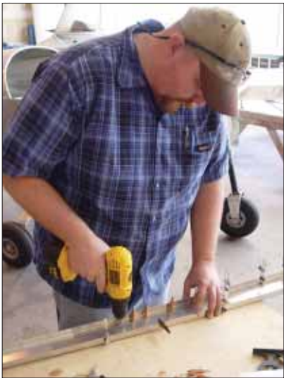
Gus Warren tackles one of the most labor-intensive parts of the fast-build kit, the rudder. You're actually expected to measure and mark holes, drill and rivet, and make a few small parts. Heresy!
