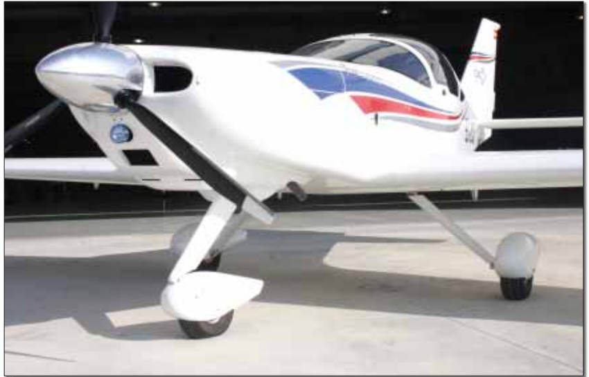
Free swiveling nosegear is standard. The main gear is a composite structure.
