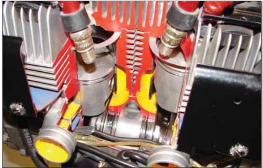
Mysteries revealed: Cutaway shows relationships among assembled parts, demonstrates how a two-stroke breathes and why internal sealing is important.
