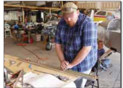
Completing the rudder in the fast-build kit is identical to what's taught at the Zenith rudder workshops. Because all operations (measuring, marking, drilling, deburring, trimming and riveting) are employed in the rudder build, overall kit progress seemed to slow a bit.
