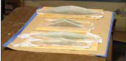
Peel-ply is all finished. Because they're on a board, we can move the parts to a warm spot in the shop and have our bench clear for another project.
