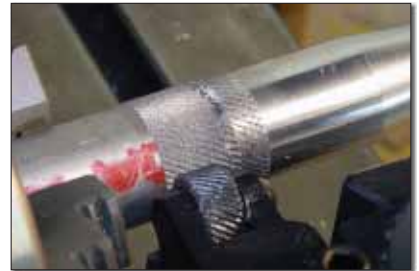
The knurl tool is simply two patterned wheels that push a pattern into the aluminum as if it were clay. Positioning the tool perpendicular to the aluminum will create a poor pattern.
