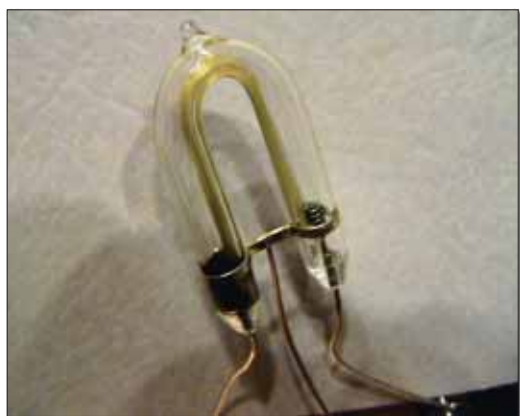
This small flashtube was used for experimentation.
