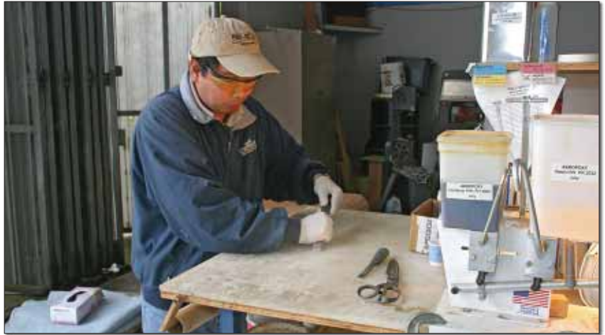
Harold Bunyi's six years at the Lancair factory shows when he emphasizes scraping the table to get the old epoxy off. He uses an ordinary wood chisel for the job.
