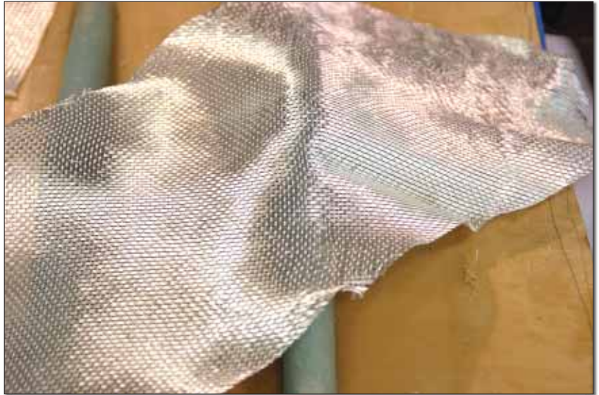
Here you can see the mold peeking out at the 6 o'clock position. Note that the threads of the fabric are also along that line, which is incorrect.
