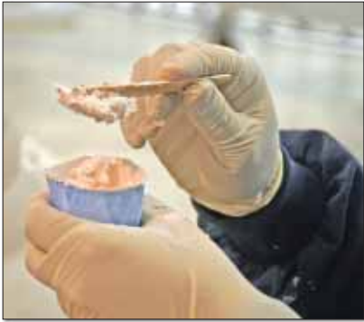
Micro and epoxy. You won't need much, and it should be pretty stiff.
