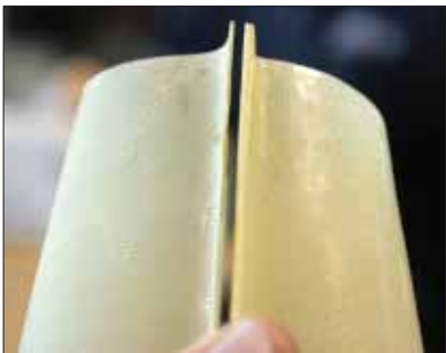
Here you can see why there is such a weight differential even though they came off of the same mold.
