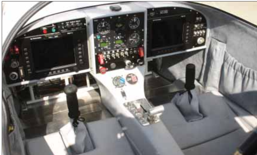
The top-of-the-line panel will use OP Technologies EFIS main displays with some steam-gauge backups.
