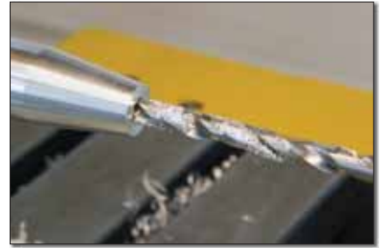
Go more than five times the diameter of the drill bit and the chips usually start to pack in the flutes. Back out, clear them away and go back in. Repeating too much takes less time than digging out broken drill bits.
