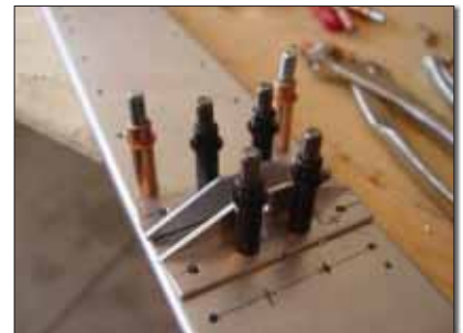
The black Clecos are for the larger 5/32-inch holes, which accept both slightly larger blind rivets or a small machine bolts. The Clecos hold two pieces precisely in place while additional holes are drilled.
