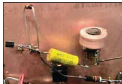
Left to right: the small black SCR, the yellow 100 nf flash capacitor, and the orange 300:6000 volt flash transformer.
