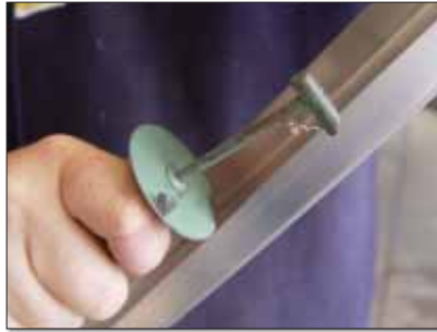
Making the freshly sheared aluminum sheets a lot safer to handle, Warren uses a different deburring tool to dull the knife-sharp edges prior to further airframe assembly.
