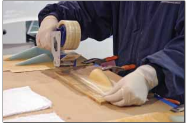
Ordinary packing tape is great for holding the mold to its base. Just remember to stay outside the boundary of the finished part.
