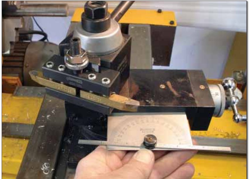
Right- and left-cutting tools are in the same holder. We're holding the protractor against the compound-slide so as to measure its angle relative to the cross-slide. The angle of the tool doesn't matter...yet.
