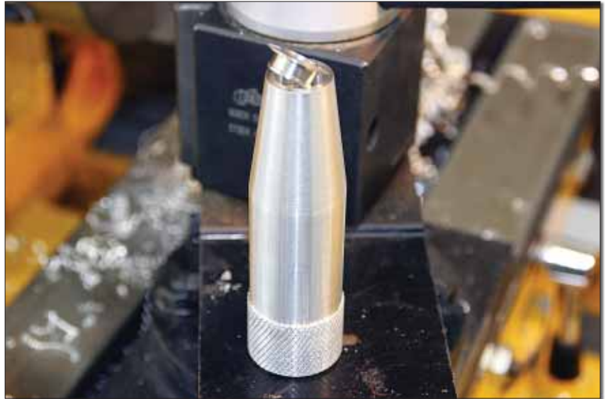
This is the finished first half of the tool with part of the cowl fastener sitting on it.
