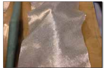
Now we've rotated the fabric 45° so that the thread lines don't cross the mold at right angles.
