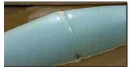
Those two shiny spots are valleys on each side of a ridge. Fill them with micro so that the shape doesn't transfer to this side of the finished part.
