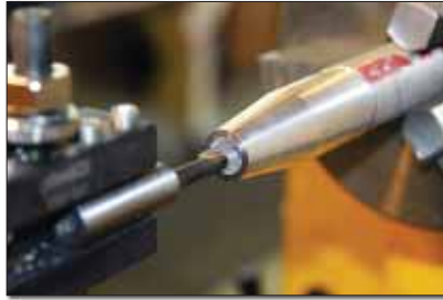
The boring tool sets up a bit differently than the other cutting tools. You have to first rotate the tool in the holder to get the cutting angle similar to that of the other tools before you set the height. Then check the clearance under the tool to make sure that the only part touching the material is the cutting edge.
