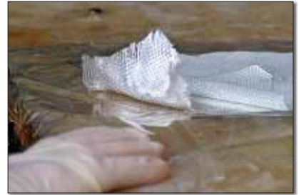
The sandwich is opened. It's two layers of cloth placed 90° to one another between two sheets of plastic wrap.
