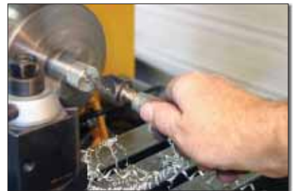
Another quickie chamfer, this time internal. The author simply put a 1-inch deburring tool into a wood handle. A quick touch, and it's done.
