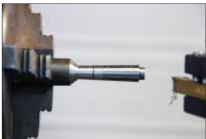
Cutting the taper this way makes it easier to cut the step.
