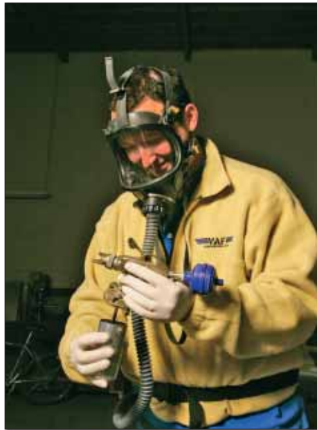
Using a spray gun—particularly for two-part epoxy primers—suggests prudence toward your health. Here, the author wears a Hobbyair forced-air respirator. Smart man!
