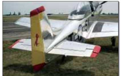
Mass- and aerodynamically balanced controls mark the T-51's tail section. The rudder and elevator are skinned in fabric, which is, as always, light and strong. Adds a period touch, too.
