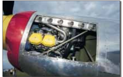
Any of the Rotax 912/914 family members will fit under the T-51's generously sized cowling. Clever use of the four-banger's exhaust helps create the something of a “poppa-poppa” short-stack sound.
