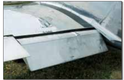
Large slotted flaps help make the T-51 docile near the ground.
