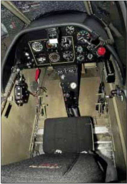
The T-51's scaled-down cockpit—from the P-51's—isn't much smaller or less comfortable. In any event, this is a sporty fun tool, not primarily a long-distance traveler.
