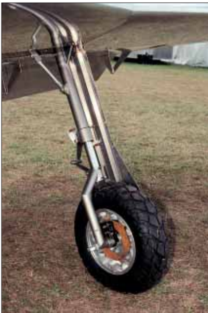
The Titan's long oleo-strutted landing gear folds inboard thanks to a hydraulic cylinder and electric power pack. These pieces are prefitted in the kit.
