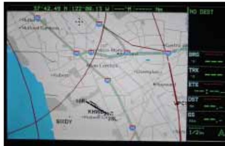
The EKP-IV also stores the flight path tracks of previous flights. Here you can see a long base entry to 28 Right.
