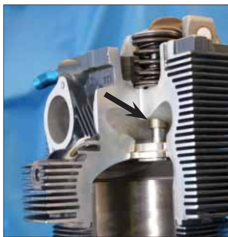
The arrow aims at the exhaust guide in a parallel-valve Lycoming head. (Actually, this is an ECI part.) It's a hard life in there, with the guide and valve stem facing high temperatures and corrosive post-combustion effluvia.
