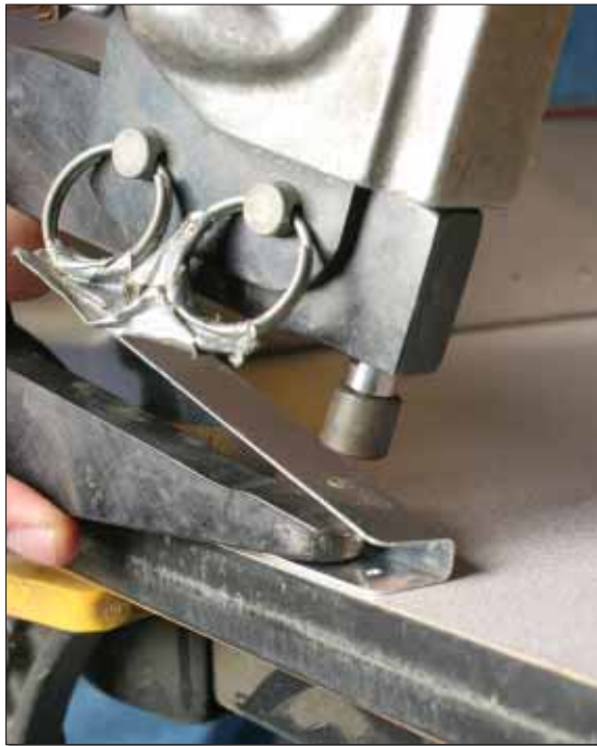
Here's where that "thin-nose no-hole" yoke comes in handy. Any other yoke style wouldn't fit in between those flanges at the trailing edge. The thin nose just fits.
