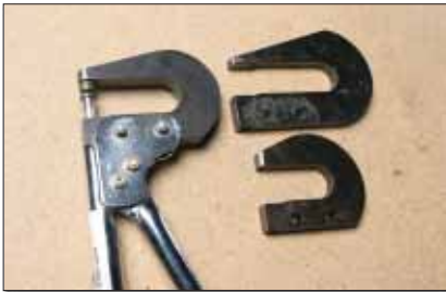
There's no end to the variety of shapes and sizes of yokes. Here are two C yokes and a "thin-nose no-hole yoke" (upper right).
