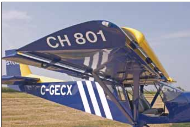
The full-span fixed slats and flaperons distinguish Zenith's STOL 801 from the typical high-wing four-seater and contribute to the low-speed characteristics of the design.
