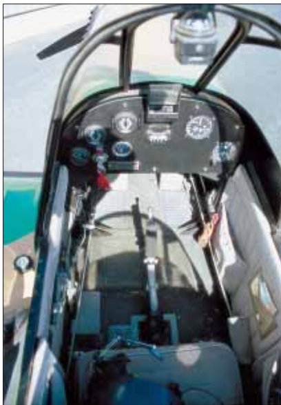
Here's the cockpit of the single-seat P-40; the red T-handle at the right is the firing pin for the BRS parachute, the handle on the stick is for brakes, and the crank and bicycle chain on the left sidewall is for gear actuation.
