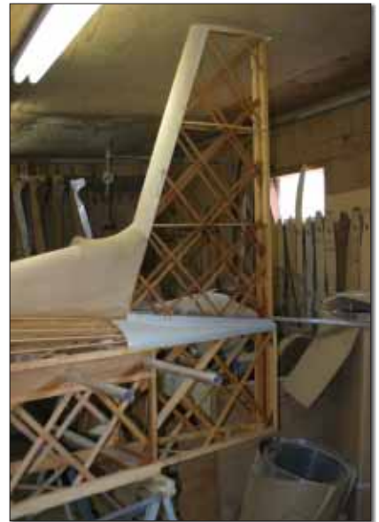
Geodetic basket-weave-arranged bracing strips provide much of the strength in the all-wood Mustang airframe.
