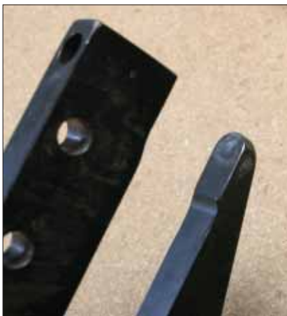
This is a close-up of the "thin-nose no-hole" yoke. You can see there's no hole at the top for a set. The top surface itself is flat and acts as the flush rivet set.
