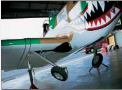
Before flying the two retractable-gear fighters, the author practiced gear retraction with the P-40 on jacks.
