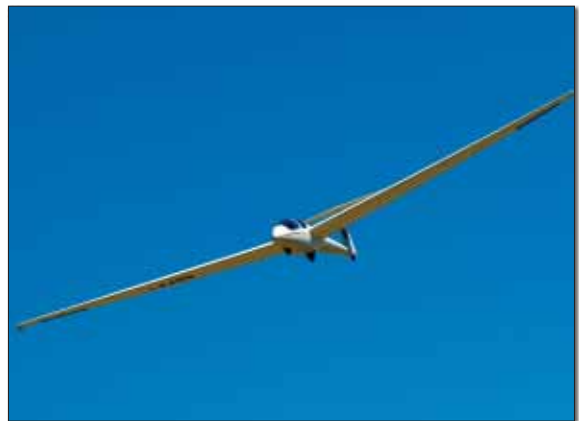
High-performance sailplanes encounter severe bending loads on their long, slender wings.
