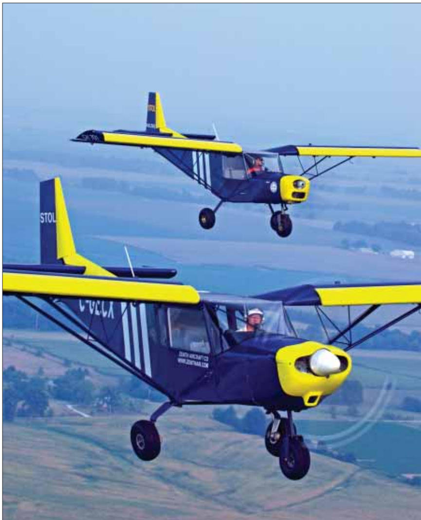
Zenith answered calls for a four-seat version of the STOL 701 (top) with the STOL 801. Heintz gave the Lycoming-powered 801 all the attributes that helped make the Rotax-powered 701 a success: the ability to launch from short fields and maneuver at very low airspeeds.
