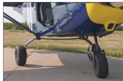
Designer Chris Heintz wanted the 801 to handle unimproved fields and firm STOL arrivals, so he designed the four-seater with a rugged one-piece leaf-spring main gear and a telescoping front strut that uses wrapped bungees to absorb shock loads.
