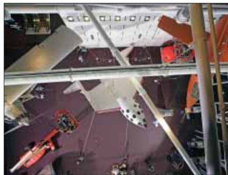
As SpaceShipOne was hoisted to its display position, the collections team took the rare opportunity to capture this overhead perspective of the gallery through the open skylights. The strongback is the white pipe running diagonally across the photo.
