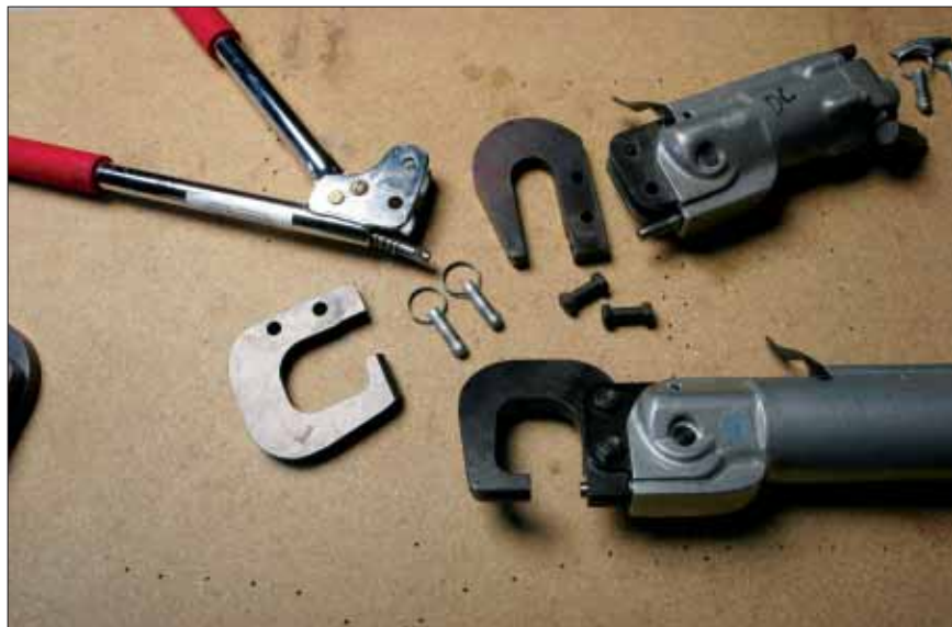
Generally, yokes are interchangeable from squeezer to squeezer—and that applies to hand and pneumatic squeezers alike. Just pull the pins (or bolts) and swap yokes.
