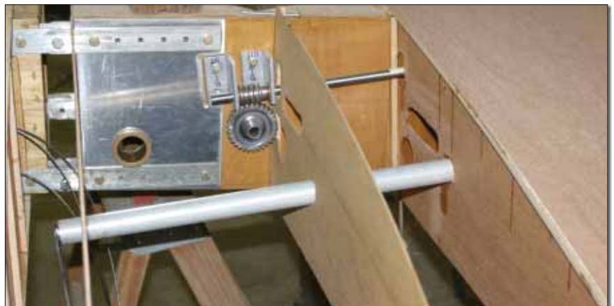
On an in-progress kit, the innards of the gear retraction system are visible. Both the Mustang and P-40 use the same system; a crank in the cockpit requires 21 turns for retraction.
