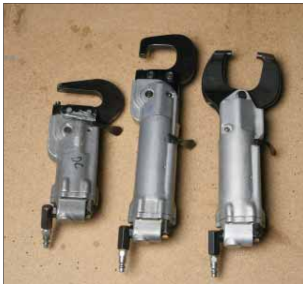
Pneumatic squeezers, from left to right: single piston, tandem piston and alligator squeezer. The tandem is capable of squeezing much larger rivets, but is often overkill.
