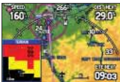
A new terrain/obstacle display on the GPSMAP 296 provides pop-up warnings of obstructions or proximity conflicts ahead.
