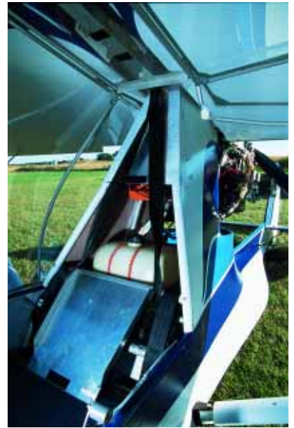
The Challenger's fuel tank rests behind the rear seat, which is folded forward in this photo.
