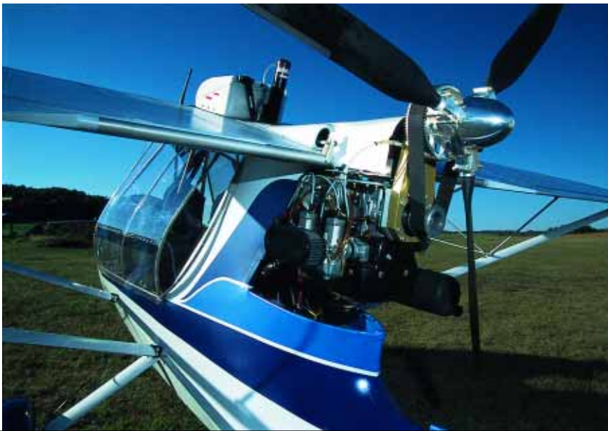
Upgrading to a Warp Drive propeller was one change Mader made during the build process.
