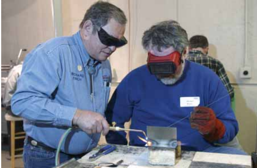
Richard Finch, who instructs EAA's course on gas welding, assists another would-be builder in the art of oxy-acetylene welding.
