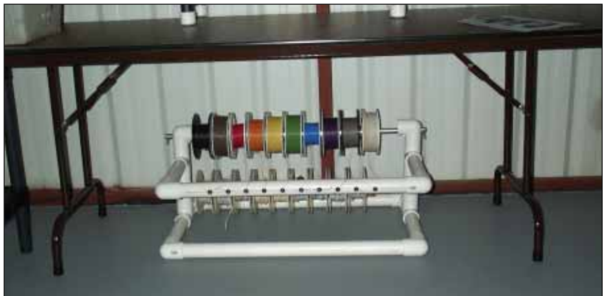
With the wire on the MK-II much lower to the ground and its frame designed as a complete box on the ground, the new wire rack can be neatly stored under a workbench in your shop.
